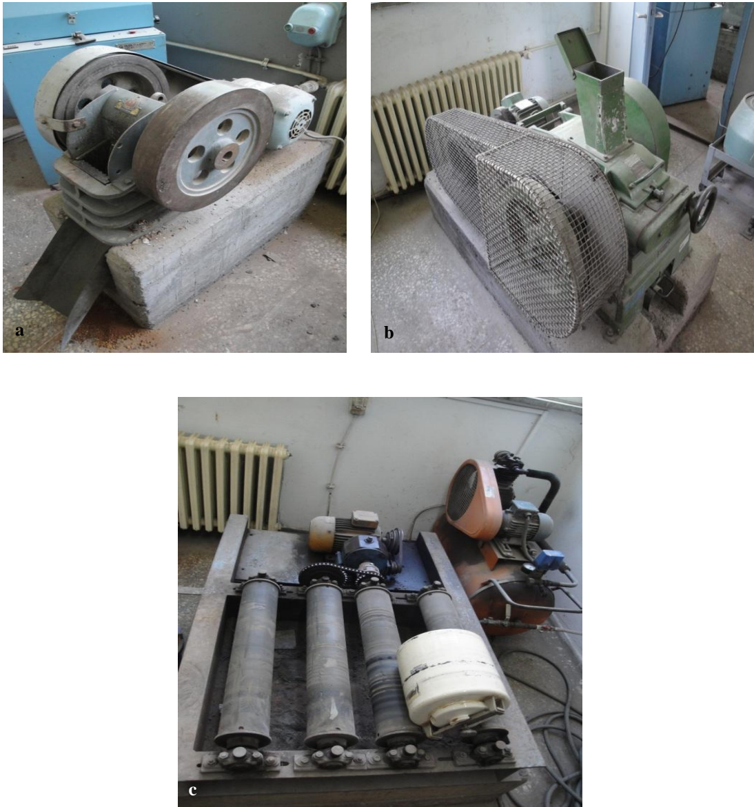
Figure 3.3 Powdering procedure, (a) breaking operation, (b) operation step 2, (c) final powdering
