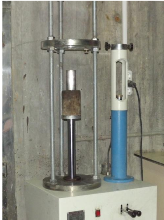
Figure 3.14 Hydraulic jack (extruding) system
