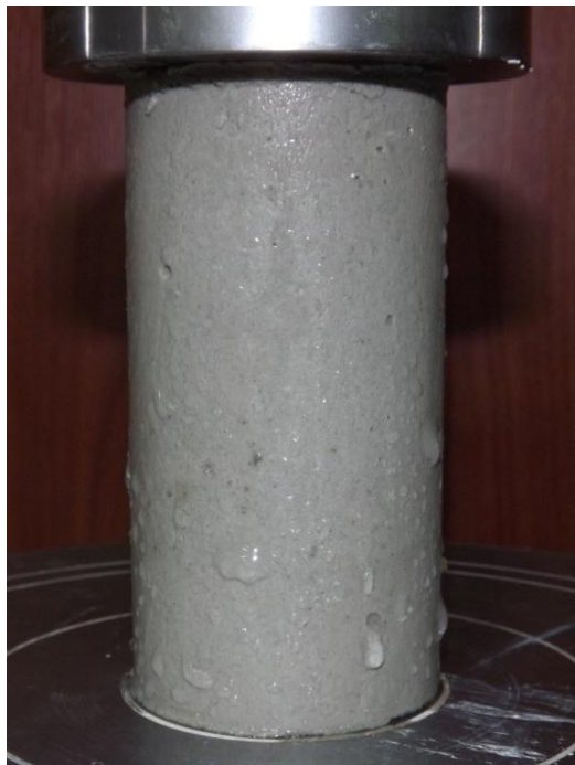
Figure 4.17 Specimen bleeding during loading
