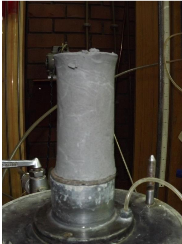
Figure 4.15 Disassembled sample after permeability test
