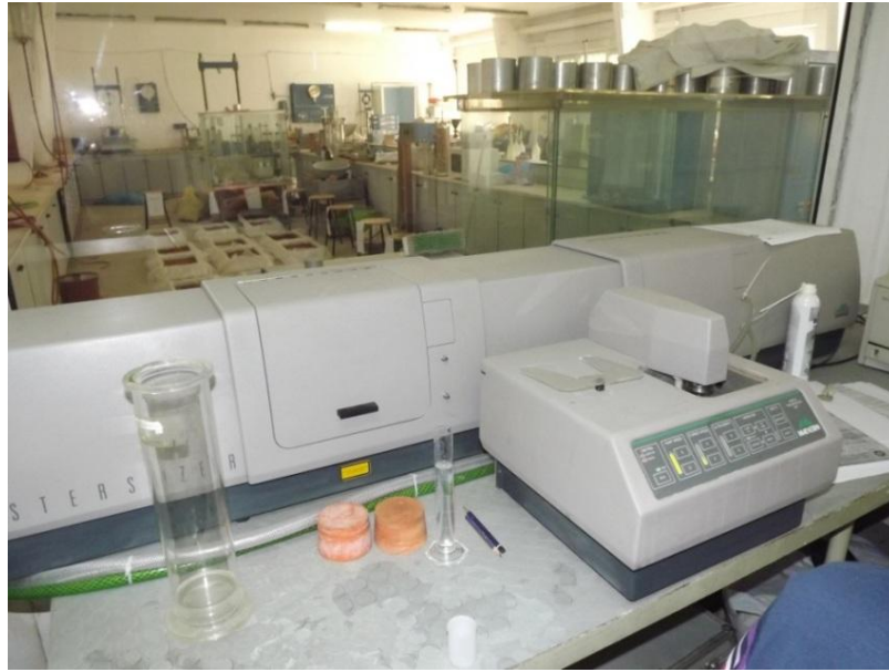
Figure 3.12 Laser Diffraction Instrument
