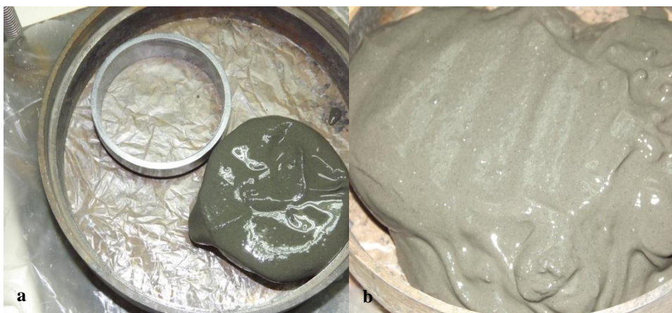
Figure 4.5 (a) Placing for consolidation cutter ring, (b) Prepared sample
