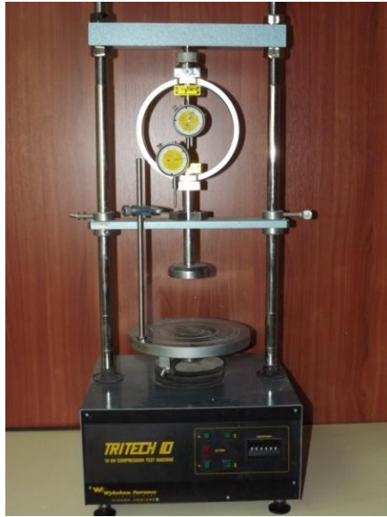
Figure 3.17 Unconfined Compressive Strength Apparatus.
