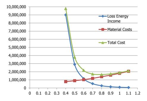
Figure 3.11 The Change in Loss Energy Income, Material Costs and Total Cost of the Penstock with respect to Diameter
