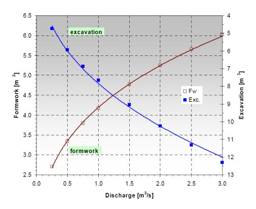
Figure A2-3 Excavation and Formwork of Conveyance Channel as a Function of Discharge
