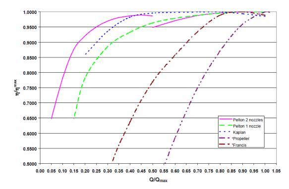
Figure 3.7 Efficiency Curves of Various Hydro Turbines (ESHA, 2004)
