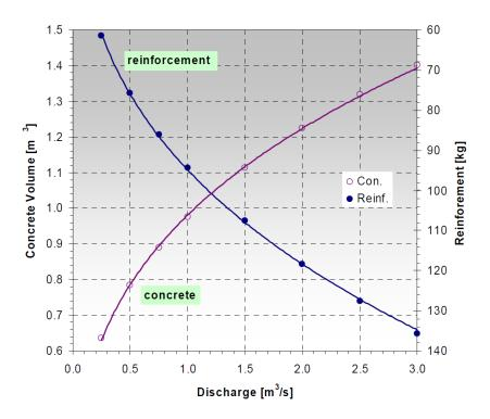
Figure A2-2 Concrete Volume and Reinforcement of Conveyance Channel as a Function of Discharge
