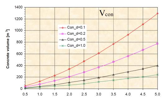
Figure A1-4 Concrete Volume of Settling Basin as a Function of Discharge and Design Grain Size as 0.1, 0.2, 0.5 and 1.0 mm
