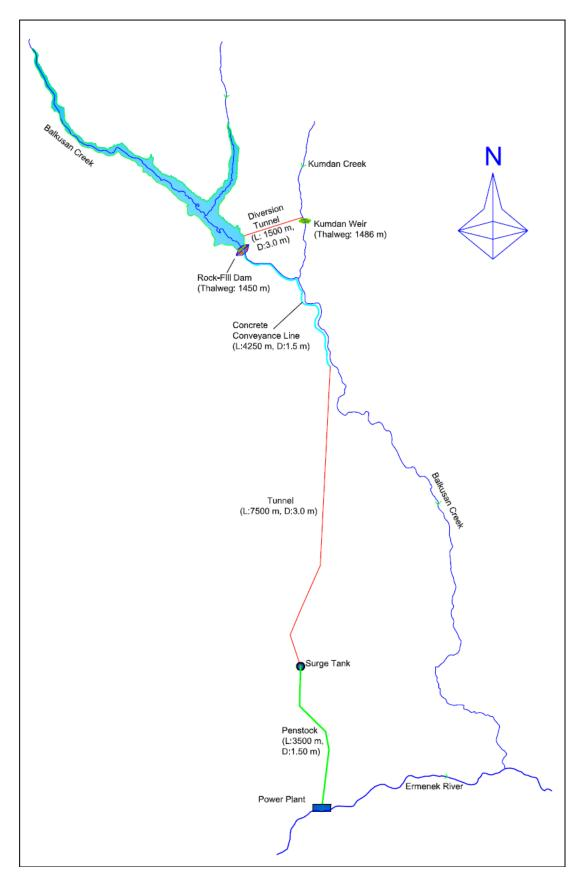
Figure 2.3 Plan of the EIEI-formulation (Not to Scale)
