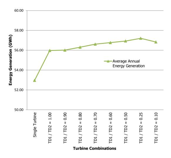
**Figure 3.16** The Change in Average Annual Energy Generation of the Discharge 2.5 m<sup>3</sup>/s with respect to Different Turbine Combinations
