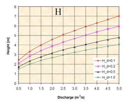
Figure A1-2 Height of Settling Basin as a Function of Discharge and Design Grain Size as 0.1, 0.2, 0.5 and 1.0 mm
