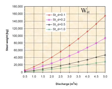
Figure A1-5 Steel Weight of Settling Basin as a Function of Discharge and Design Grain Size as 0.1, 0.2, 0.5 and 1.0 mm
