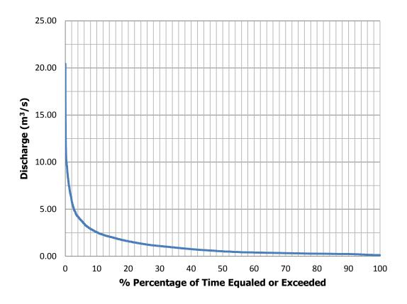
Figure 3.5 Flow-duration Curve of the Alternative-formulation
