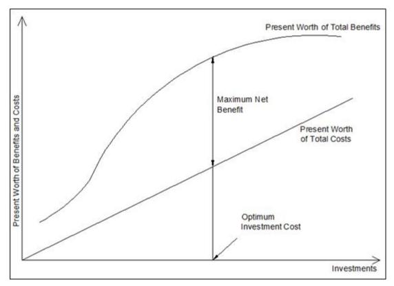
Figure 3.1. Cost and Income versus Installed Capacity Chart for Water Resources Investments (Karataban, 1976)
