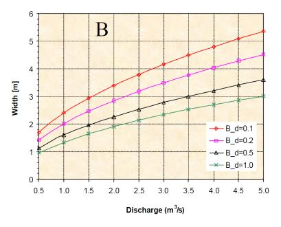
Figure A1-1 Width of Settling Basin as a Function of Discharge and Design Grain Size as 0.1, 0.2, 0.5 and 1.0 mm
