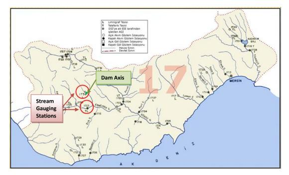
Figure 2.11 Locations of Dam Axis, EIEI 1736 and EIEI 1723 Stream Gauging Stations
