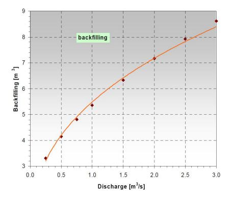
Figure A2-4 Backfilling of Conveyance Channel as a Function of Discharge
