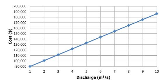
Figure 3.13 Forebay Cost as a Function of Discharge (EIEI, 2006)
