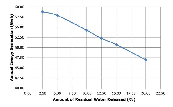
Figure 3.15 The Change in Annual Energy Generation as a Function of Residual Water
