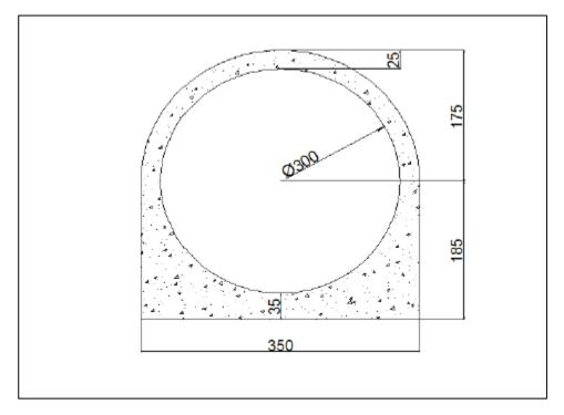
Figure 3.12 Tunnel Cross-Section (All dimensions are in cm) (Hidromark, 2009)
