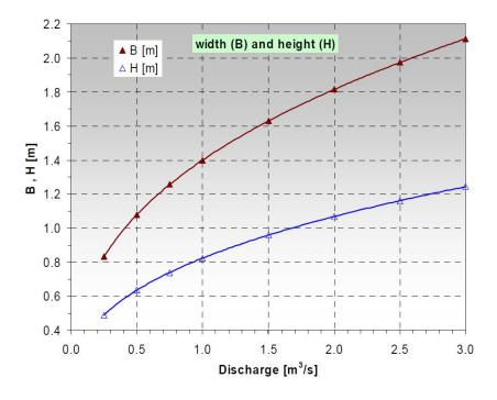
Figure A2-1 Width and Height of Conveyance Channel as a Function of Discharge
