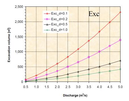
Figure A1-6 Excavation Volume of Settling Basin as a Function of Discharge and Design Grain Size as 0.1, 0.2, 0.5 and 1.0 mm
