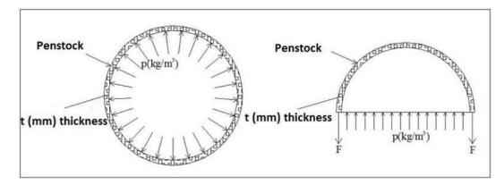
Figure 3.10 Penstock Cross-Section and the Forces and Pressures on it (Calamak, 2010)
