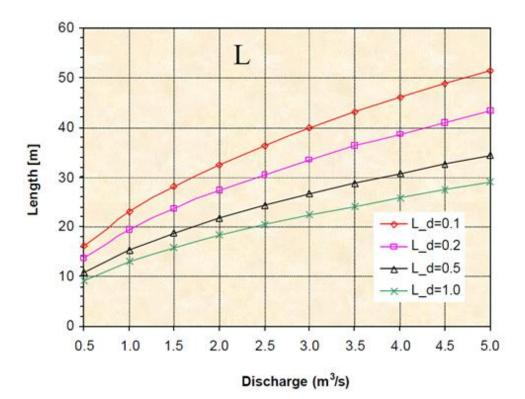
Figure A1-3 Length of Settling Basin as a Function of Discharge and Design Grain Size as 0.1, 0.2, 0.5 and 1.0 mm
