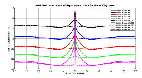
Figure 42: Vertical Displacement during 25 %, 40 %, 55 %, 70 % and 85 % of Consolidation Process at the Depth of 5 m
