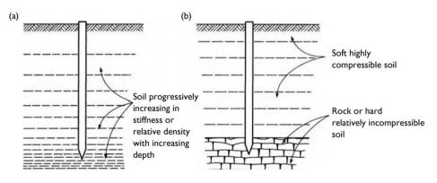
Figure 1: Types of bearing pile (a) Friction pile (b) End - bearing pile (Tomlinson and Woodward, 2008)
