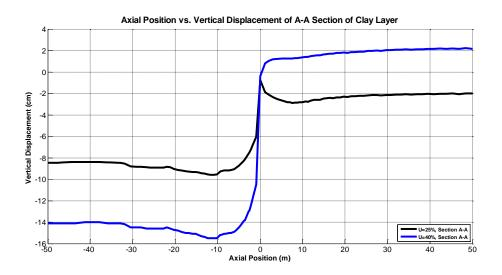
Figure 52: Vertical Displacement during 25 % and 40 % of Consolidation Process at the Depth of 5 m
