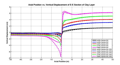
Figure 64: Vertical Displacement during 25 %, 40 %, 55 %, 70 % and 85 % of Consolidation Process at the Depth of 11 m
