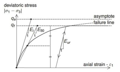
Figure 23: Hyperbolic Stress-Strain Relation in Primary Loading for a Standard Drained Triaxial Test (PLAXIS 2D User's Manual, 2010)
