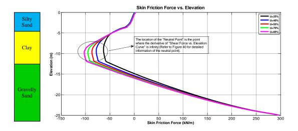
Figure 39: Skin Friction Force Acting on the Wall as a Function of Vertical Position of the Wall
