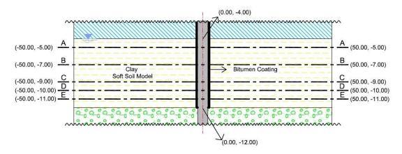
Figure 41: The Axial Sections of the Clay Layer
