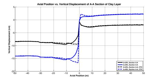
Figure 61: Vertical Displacement during 25 % and 40 % of Consolidation Process at the Depth of 5 m
