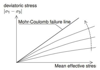
Figure 24: Successive Yield Loci for Various Constant Values of the Hardening Parameter γ<sup>p</sup> (PLAXIS 2D User's Manual, 2010)
