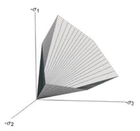
Figure 19: The Mohr - Coulomb Yield Surface In Principal Stress Space (c=0) (PLAXIS 2D User's Manual, 2010)
