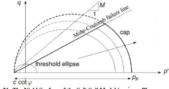
Figure 21: The Yield Surface of the Soft Soil Model in p' - q Plane
