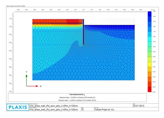
Figure B 9: Total Displacements (u<sub>y</sub>) (Step 5)
