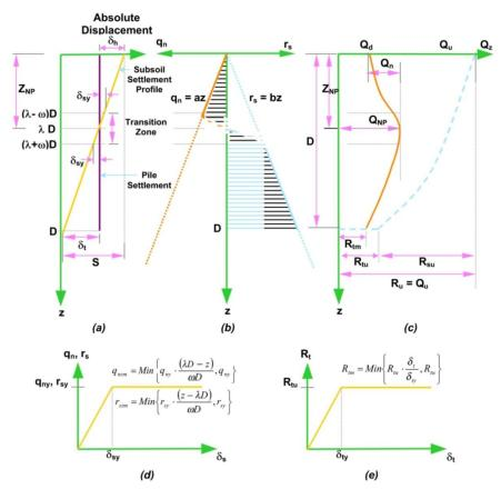
Figure 6: Negative Skin Friction on a Single Pile (Elastic Plastic Model) (Shong, 2002)
