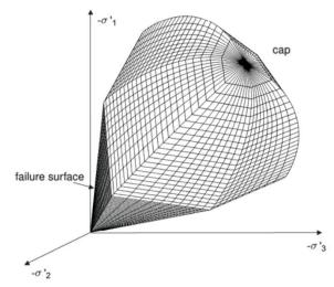
Figure 22: Representation of the Total Yield Contour of the Soft Soil Model in Principal Stress Space (PLAXIS 2D User's Manual, 2010)
