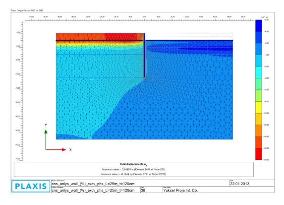
Figure B 6: Total Displacements (u<sub>y</sub>) (Step 4)
