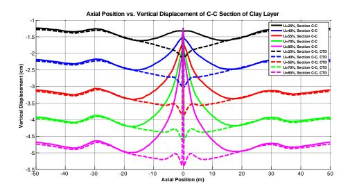
Figure 44: Vertical Displacement during 25 %, 40 %, 55 %, 70 % and 85 % of Consolidation Process at the Depth of 9 m
