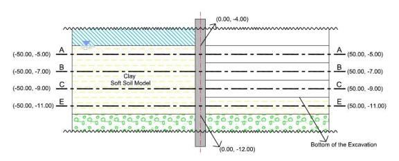
Figure 51: The Axial Sections of the Clay Layer
