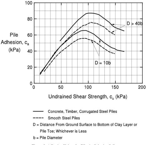
Figure 8: Adhesion Values for Piles in Cohesive Soil (Design and Construction of Driven Pile Foundations, 1998)
