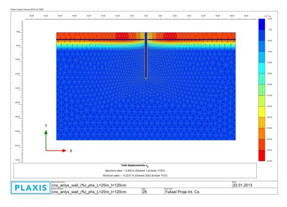
Figure A 7: Total Displacements (u<sub>y</sub>) (Step 5)
