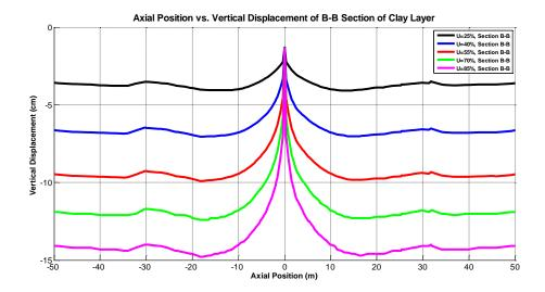
Figure 33: Vertical Displacement during 25 %, 40 %, 55 %, 70 % and 85 % of Consolidation Process at the Depth of 7 m
