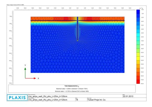
Figure A 5: Total Displacements (u<sub>y</sub>) (Step 4)
