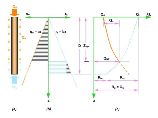
Figure 5: Negative Skin Friction on a Single Pile (Rigid Plastic Model) (L. Shaw Shong, 2002)
