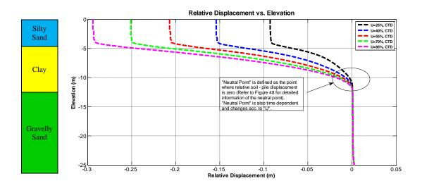
Figure 47: Relative Displacement of the Wall and the Soil
