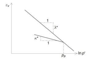
Figure 20: Logarithmic Relation Between Volumetric Strain and Mean Stress (PLAXIS 2D User's Manual, 2010)
