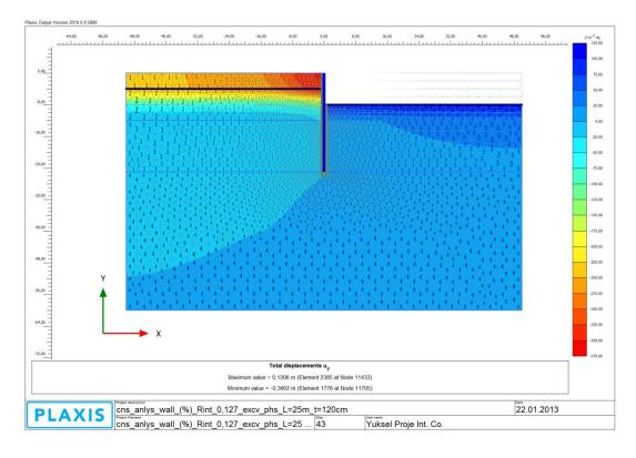
Figure B 28: Total Displacements (u<sub>y</sub>) (Step 6)
