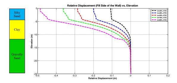
Figure 65: Relative Displacement of the Fill Side of the Wall and the Soil
