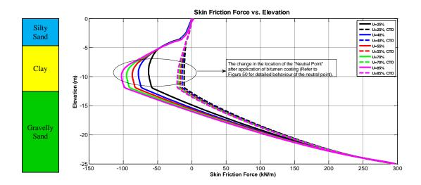
Figure 49: Skin Friction Force Acting on the Wall as a Function of Vertical Position of the Wall
