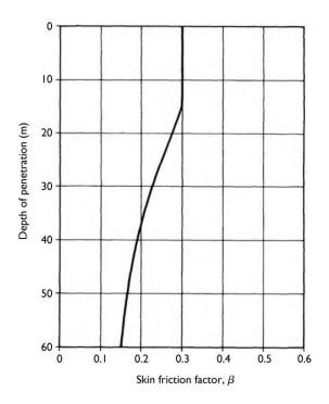
Figure 9: Negative Skin Friction Factors for Piles Driven into Soft to Firm Clays (Tomlinson and Woodward, 2008)
