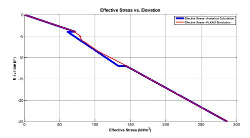
Figure 77: Comparison of Effective Stress Calculation of PLAXIS<sup>TM</sup> Simulation and the Analytical Method Utilized
