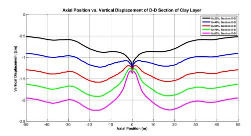
Figure 35: Vertical Displacement during 25 %, 40 %, 55 %, 70 % and 85 % of Consolidation Process at the Depth of 10 m
