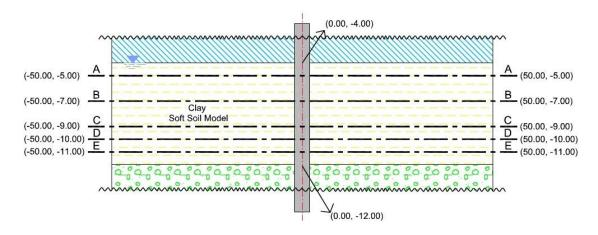
Figure 31: Selected Axial Cross Sections of the Clay Layer
