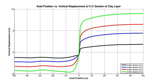
Figure 54: Vertical Displacement during 25 %, 40 %, 55 % and 70 % of Consolidation Process at the Depth of 9 m
