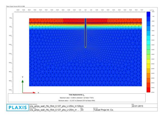
Figure A 22: Total Displacements (u<sub>y</sub>) (Step 7)
