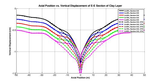
Figure 46: Vertical Displacement during 25 %, 40 %, 55 %, 70 % and 85 % of Consolidation Process at the Depth of 11 m
