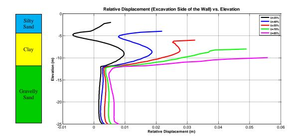
Figure 57: Relative Displacement of the Excavation Side of the Wall and the Soil
