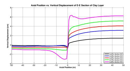
Figure 55: Vertical Displacement during 25 %, 40 %, 55 %, 70 % and 85 % of Consolidation Process at the Depth of 11 m
