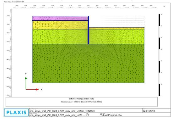
Case 2: Bitumen Coated Diaphragm Wall - Soil Interaction Model during Excavation
