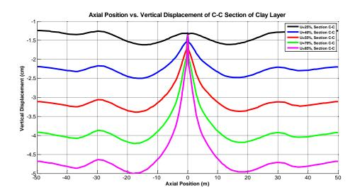
Figure 34: Vertical Displacement during 25 %, 40 %, 55 %, 70 % and 85 % of Consolidation Process at the Depth of 9 m
