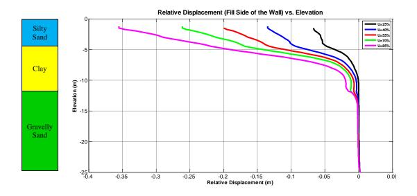
Figure 56: Relative Displacement of the Fill Side of the Wall and the Soil
