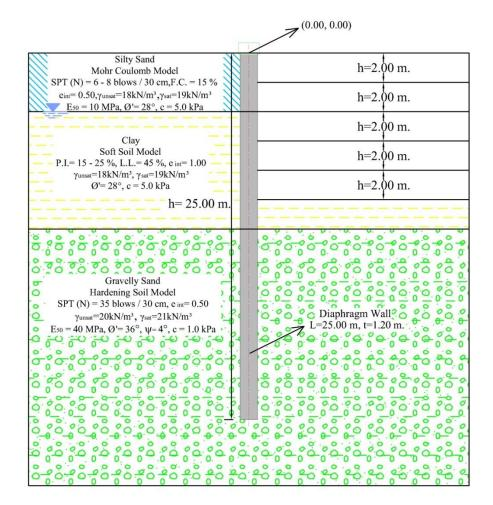
Figure 28: Diaphragm Wall Application And Excavation Of The Site
