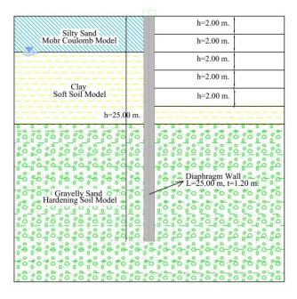
Figure 14: The Excavation Process (2.00 meters of Excavation at Each Step)
