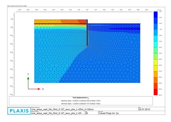
Figure B 22: Total Displacements (u<sub>y</sub>) (Step 4)
