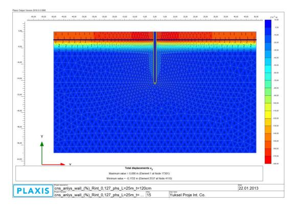
Figure A 16: Total Displacements (u<sub>y</sub>) (Step 4)
