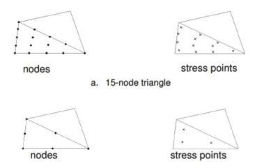
Figure 17: Position of Nodes and Stress Points in Soil Elements (PLAXIS 2D User's Manual, 2010)
