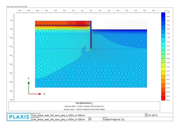
Figure B 12: Total Displacements (u<sub>y</sub>) (Step 6)
