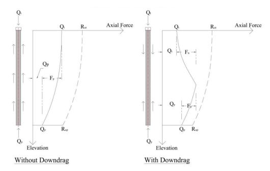
Figure 2: Distribution of Axial Forces in a Pile (Briaud & Tucker, 1996)
