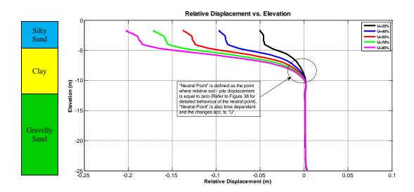
Figure 37: Relative Displacement of the Wall and the Soil
