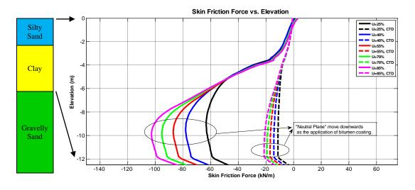
Figure 50: The Behavior of the Skin Friction Force Acting on the Wall around the Neutral Point
