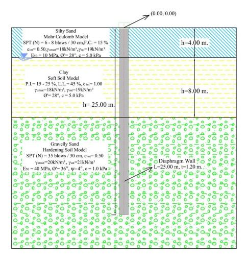
Figure 25: The Geological Profile of the Analyzed Soil Section
