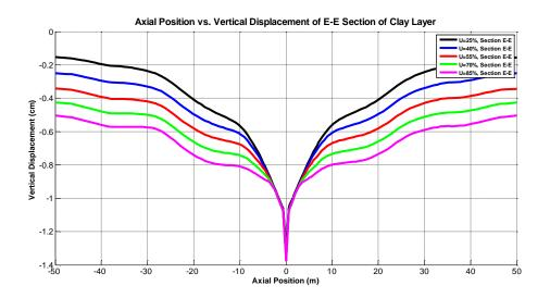
Figure 36: Vertical Displacement during 25 %, 40 %, 55 %, 70 % and 85 % of Consolidation Process at the Depth of 11 m
