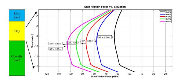
Figure 40: The Behavior of the Skin Friction Force Acting on the Wall around the Neutral Point
