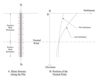
Figure 3: Negative Skin Friction on a Pile (Briaud & Tucker, 1996)
