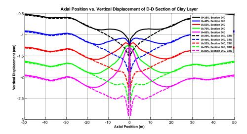
Figure 45: Vertical Displacement during 25 %, 40 %, 55 %, 70 % and 85 % of Consolidation Process at the Depth of 10 m
