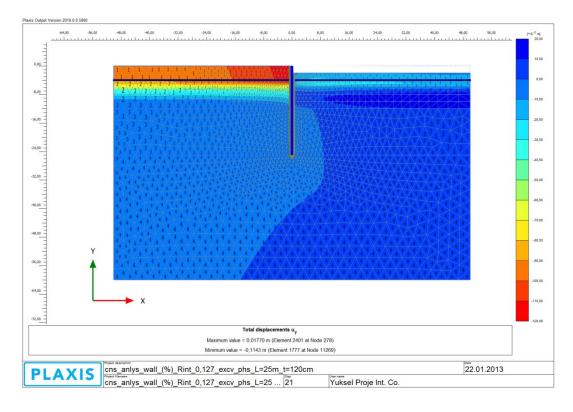
Figure B 19: Total Displacements (u<sub>y</sub>) (Step 3)
