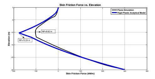
Figure 78: Comparison of Skin Friction Force Calculation of PLAXIS<sup>TM</sup> Simulation and the Analytical Method Utilized (Simplified)
