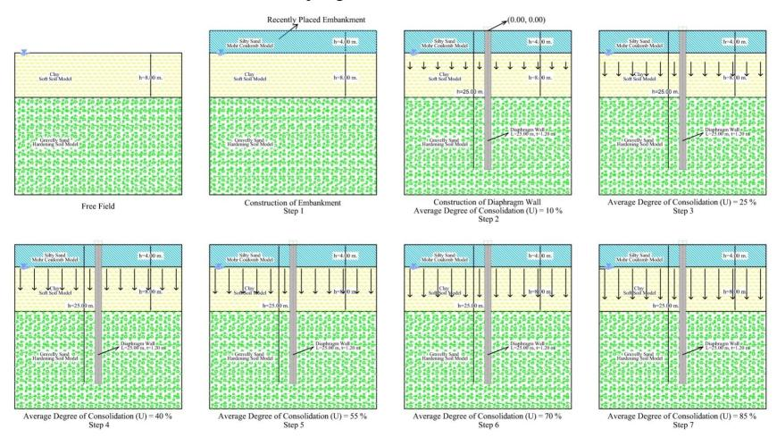
Figure 26: The Sequence of Events for Pure Consolidation Assessment
