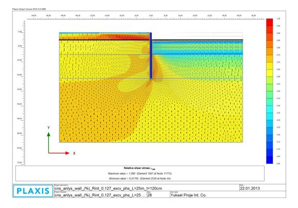
Figure B 23: Relative Shear Stress (**trel**) (Step 4)
