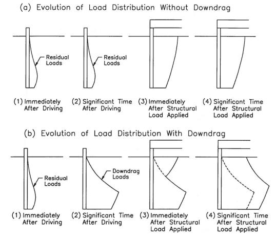
Figure 10: Evolution of the Load Distribution in a Pile (Briaud & Tucker, 1996)
