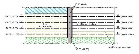
Figure 60: The Axial Sections of the Clay Layer
