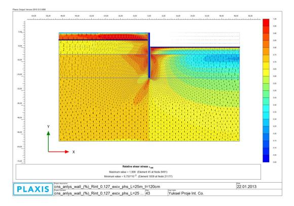
Figure B 29: Relative Shear Stress (**trel**) (Step 6)
