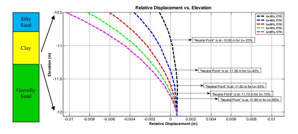
Figure 48: Relative Displacement of the Wall and the Soil Close to Neutral Point
