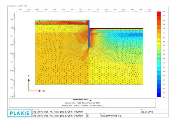
Figure B 13: Relative Shear Stress (**trel**) (Step 6)
