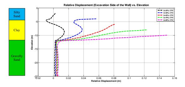
Figure 66: Relative Displacement of the Excavation Side of the Wall and the Soil
