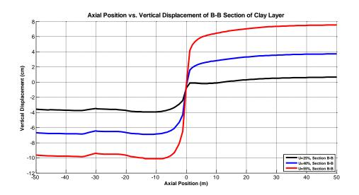
Figure 53: Vertical Displacement during 25 %, 40 % and 55 % of Consolidation Process at the Depth of 7 m
