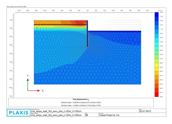
Figure B 15: Total Displacements (u<sub>y</sub>) (Step 7)
