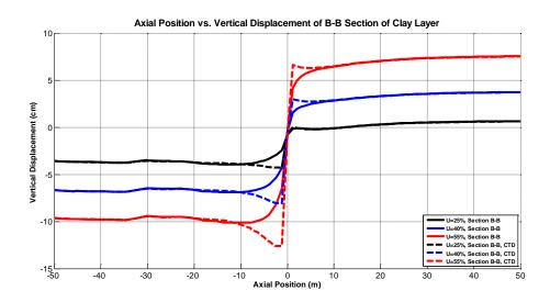
Figure 62: Vertical Displacement during 25 %, 40 % and 55 % of Consolidation Process at the Depth of 7 m
