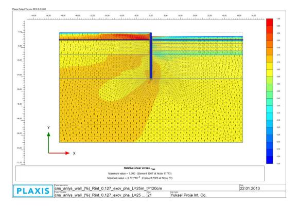
Figure B 20: Relative Shear Stress (**trel**) (Step 3)
