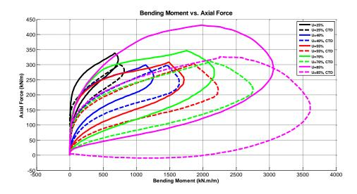
Figure 73: Bending Moment vs. Axial Force Characteristics for Simulation Steps 3, 4, 5, 6 and 7
