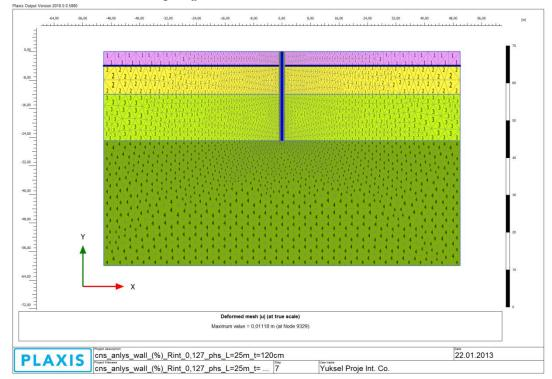
Case 2: Bitumen Coated Diaphragm Wall - Soil Interaction Model
