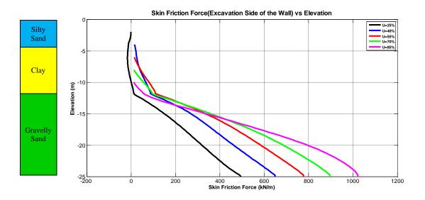
Figure 59: Skin Friction Force Acting on the Excavation Side of the Wall as a Function of Vertical Position of the Wall
