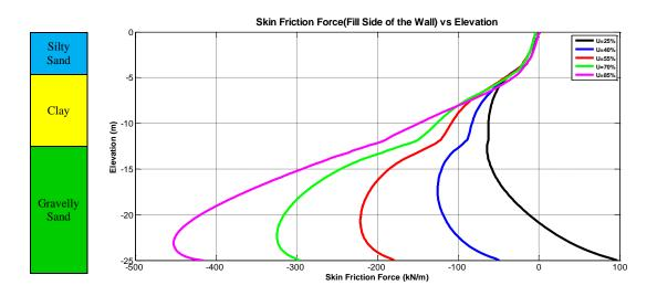
Figure 58: Skin Friction Force Acting on the Fill Side of the Wall as a Function of Vertical Position of the Wall
