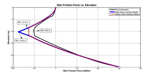
Figure 79: Comparison of Skin Friction Force Calculation of PLAXIS<sup>TM</sup> Simulation and the Analytical Method Utilized
