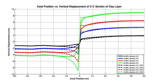
Figure 63: Vertical Displacement during 25 %, 40 %, 55 % and 70 % of Consolidation Process at the Depth of 9 m
