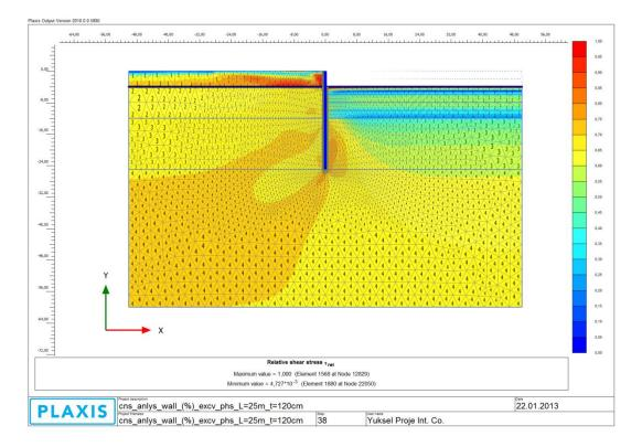
Figure B 7: Relative Shear Stress (**trel**) (Step 4)
