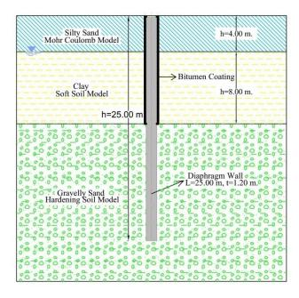
Figure 13: Application of Bitumen Coating
