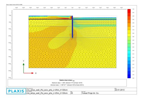
Figure B 4: Relative Shear Stress (**trel**) (Step 3)
