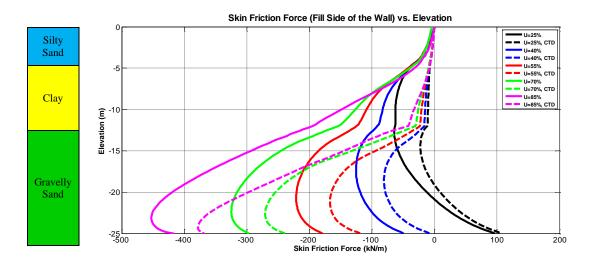
Figure 67: Skin Friction Force Acting on the Fill Side of the Wall as a Function of Vertical Position of the Wall
