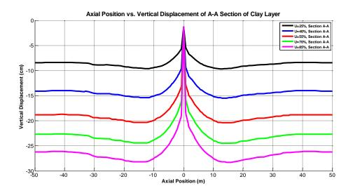
Figure 32: Vertical Displacement during 25 %, 40 %, 55 %, 70 % and 85 % of Consolidation Process at the Depth of 5 m
