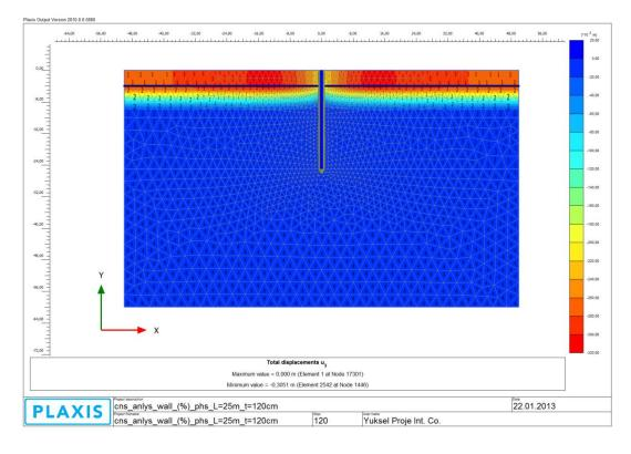
Figure A 11: Total Displacements (u<sub>y</sub>) (Step 7)
