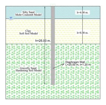
Figure 12: Construction of Diaphragm Wall
