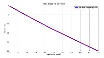
Figure 75: Comparison of Total Stress Calculation of PLAXIS<sup>TM</sup> Simulation and the Analytical Method Utilized
