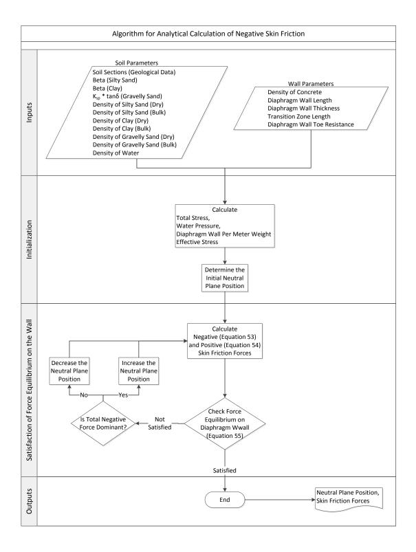
Figure 74: Flowchart for Analytical Negative Skin Friction Calculation Algorithm
