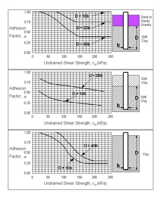
Figure 7: Adhesion factors for Driven Piles in Clay (Design and Construction of Driven Pile Foundations, 1998)
