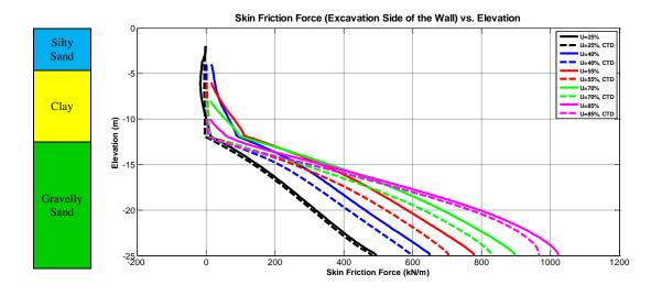
Figure 68: Skin Friction Force Acting on the Excavation Side of the Wall as a Function of Vertical Position of the Wall
