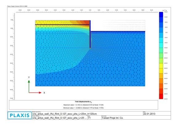
Figure B 31: Total Displacements (u<sub>y</sub>) (Step 7)
