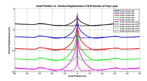
Figure 43: Vertical Displacement during 25 %, 40 %, 55 %, 70 % and 85 % of Consolidation Process at the Depth of 7 m
