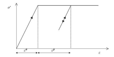
Figure 18: The Basic Idea of an Elastic Perfectly Plastic Model (PLAXIS 2D User's Manual, 2010)
