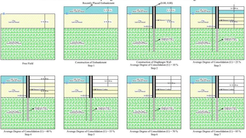
Case 2: Bitumen Coated Diaphragm Wall - Soil Interaction Model during Excavation
