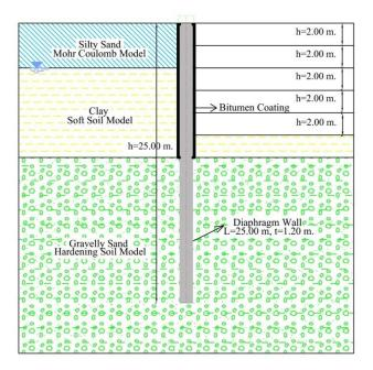
Figure 15: Application of Bitumen Coating
