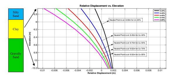
Figure 38: Relative Displacement of the Wall and the Soil Close to Neutral Point
