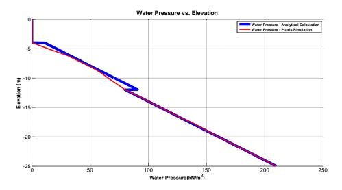
Figure 76: Comparison of Water Pressure Calculation of PLAXIS<sup>TM</sup> Simulation and the Analytical Method Utilized
