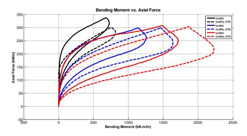
Figure 71: Bending Moment vs. Axial Force Characteristics for Simulation Steps 3, 4 and 5
