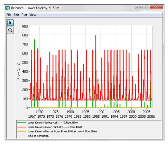
Figure 3.33 Graphical display of "Releases plot" function
