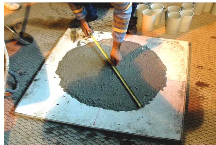
Figure 3.9 Slump flow test method
