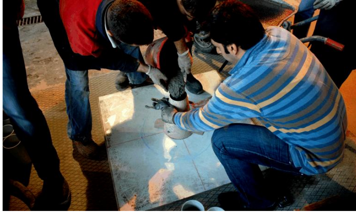
Figure 3.7 Slump and T500 test method for fresh SCC
