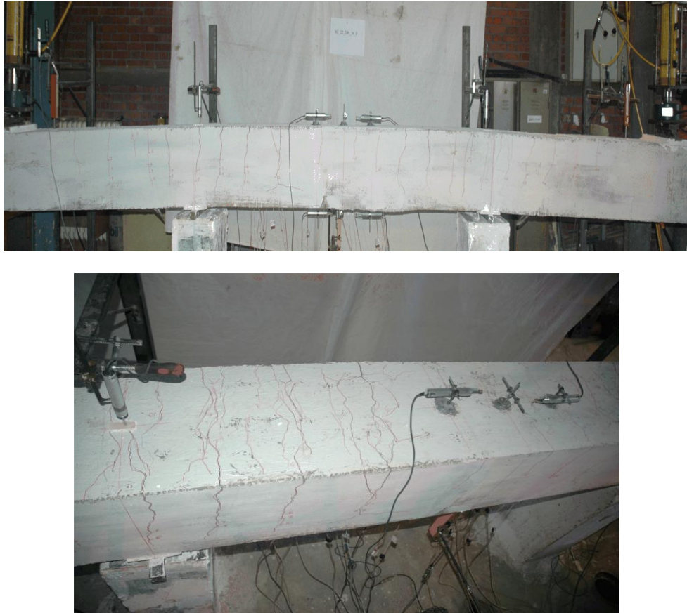
Figure 4.11 Cracks formation on the side and bottom cover of the specimen
