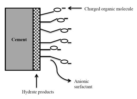
Figure 1.14 Adsorption of the charged organic molecules on the cement particles.
