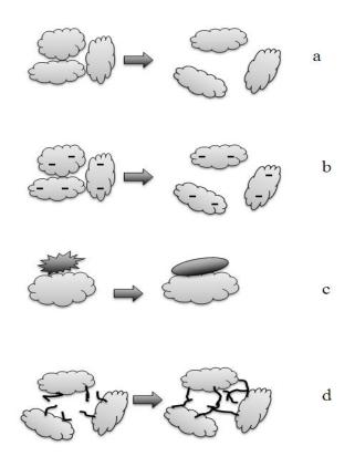
Figure 1.17 Effects of plasticizers on concrete and cement particles. a) creating a grease layer, b) surrounding the particles and giving negative charges, c) decreasing water's surface tension d) creating long polymer chains (Lazinewska – Piekarczyk, 2012).
