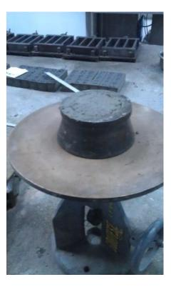
Figure 2.3 Flow table with the concrete mold.
