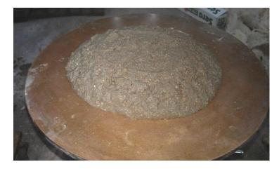
Figure 2.7 Concrete mixture with cotton stalk lignin after flow.
