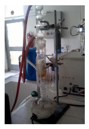
Figure 2.1 The extraction setup.
