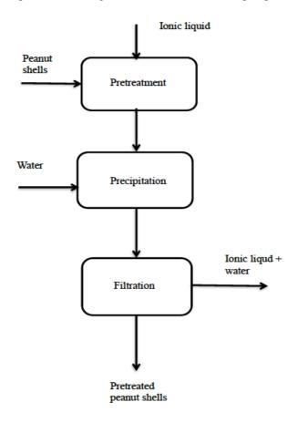
Figure 3.14 Flow diagram of ionic liquid pretreatment.
