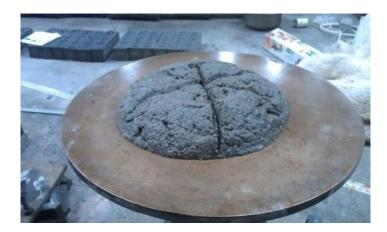
Figure 2.5 Control mix after flow.
