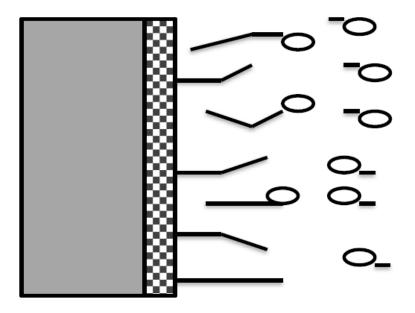
Figure 1.16 Film formation at cement particle – solution interface.
