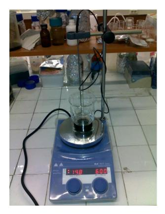
Figure 2.2 Experimental setup for the ionic liquid pretreatments.
