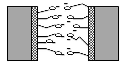
Figure 1.15 Steric and electrostatic particle – particle repulsion.
