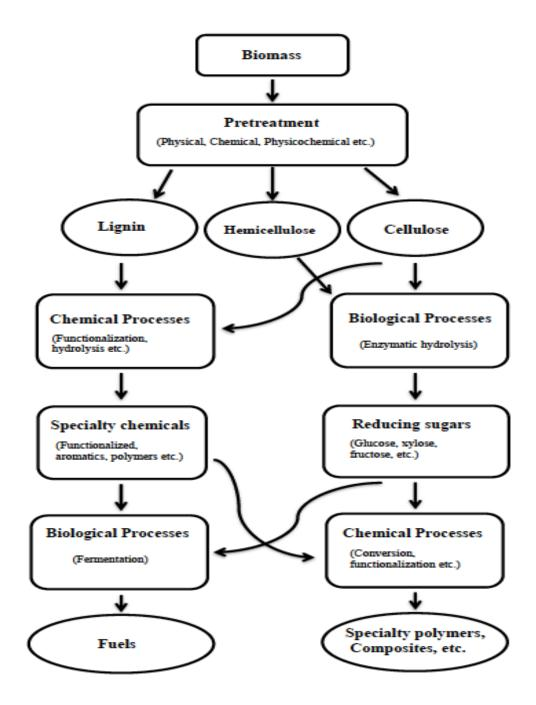
Figure 1.1 Schematic of biorefinery concept (FitzPatrick et al., 2010).
