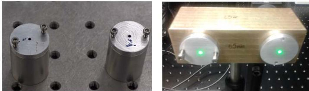
**Figure 45** Pinholes for objective alignment
