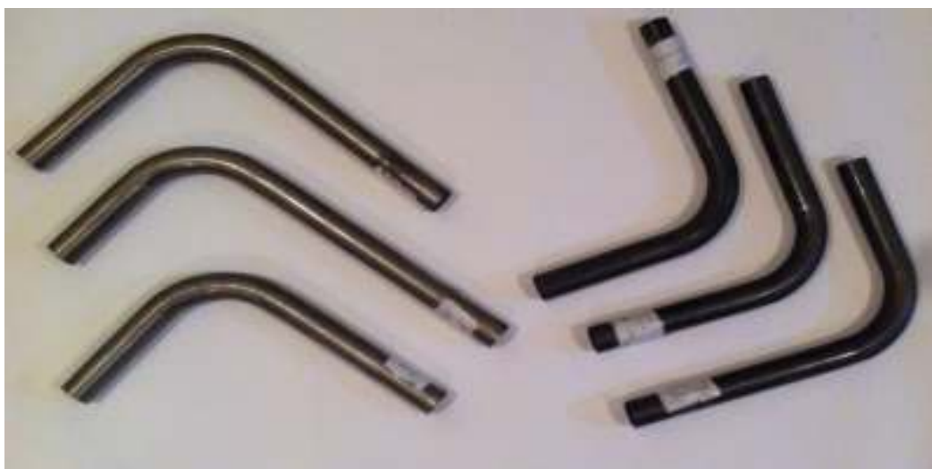
Figure 4-9 Bent Tubes Used in Finding the Optimum Seam Position
