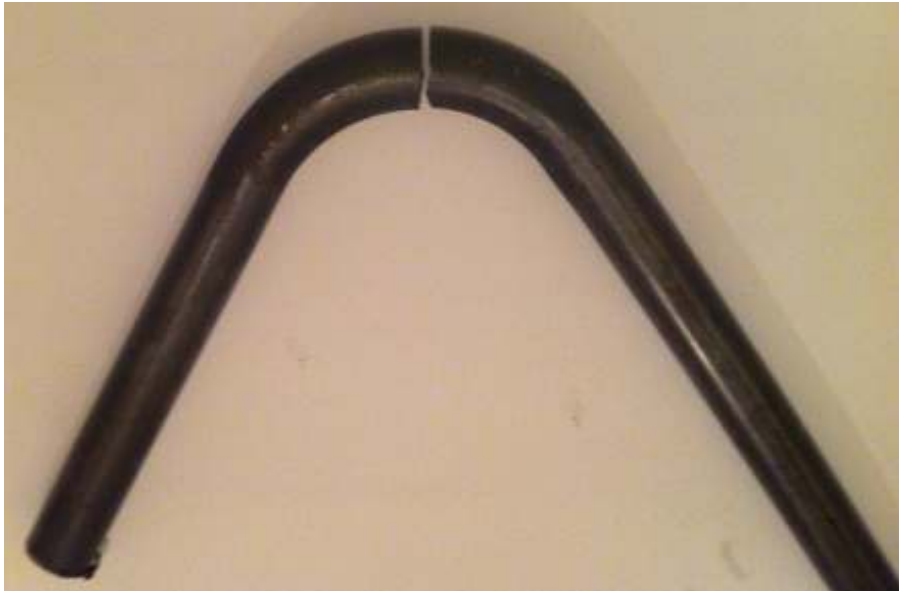
Figure 4-12 A 120° bent St37 Steel Tube Cut after Bending Operation
