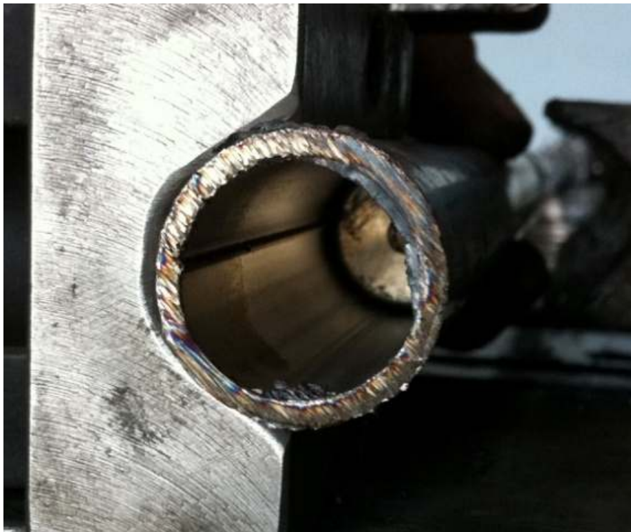
Figure 4-7 Seam of the Tube at the Compression Side
