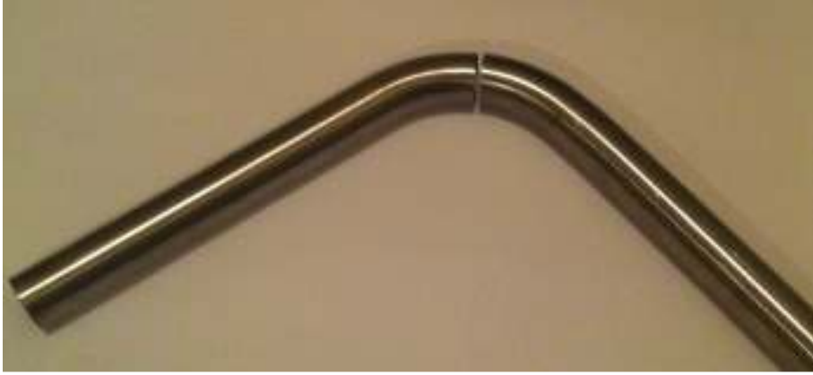
Figure 4-11 A 90° Bent SS304 Stainless Steel Tube Cut after Bending Operation
