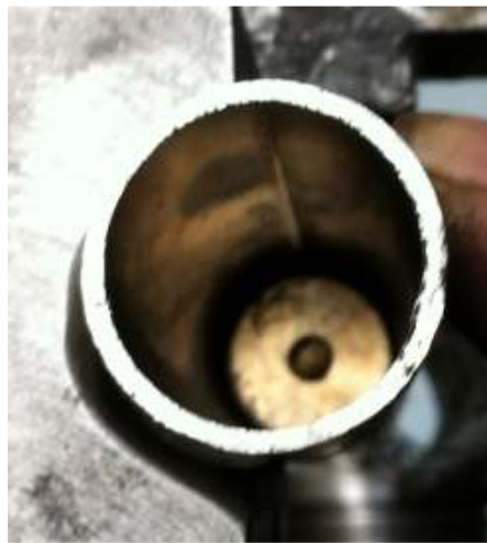
Figure 4-8 Seam is placed at the Upper Side
