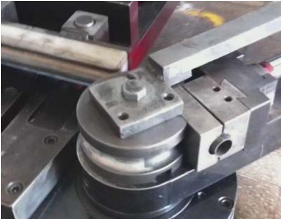
Figure 4-5 Rotary Draw Bending Operation
