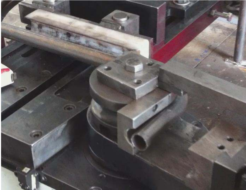
Figure 4-6 Unloading of the Pressure Die and Clamp Die and Initialization of Spring-Back
