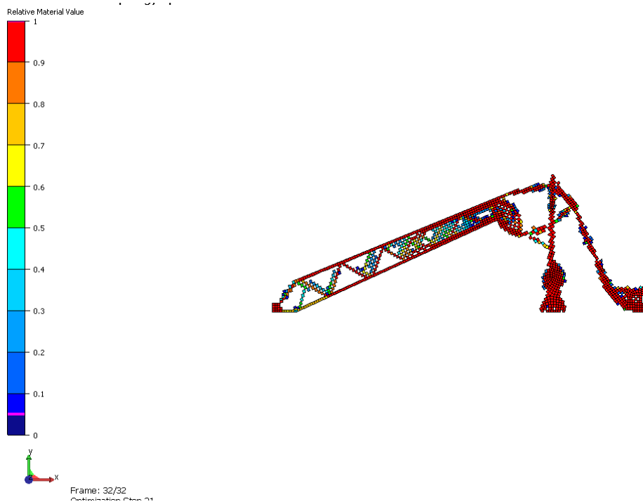
Figure 10 Displacement response for the final configuration of the topology optimization run (first lever section part of the compliant mechanism)
