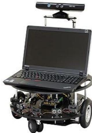
Figure 4 - Parallax Eddie Robot Platform [4]
