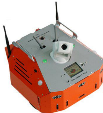
Figure 7 - Dr. Robot Sentinel3 Wi-Fi Mobile Development Platform [7]
