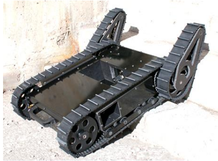
Figure 8 - Dr. Robot Jaguar Tracked Mobile Platform [8]
