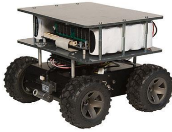
Figure 10 - CoroWare CoroBot CB-W Robot Development Platform [10]
