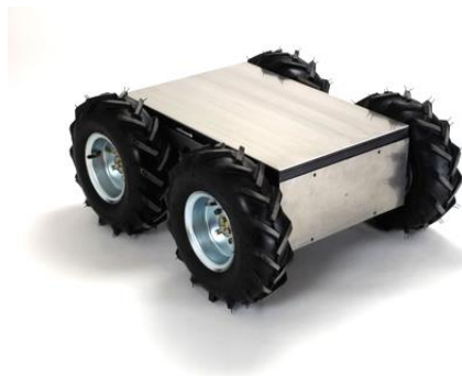
Figure 9 - InspectorBots Mega Bot Wireless 4WD Robot Platform [9]
