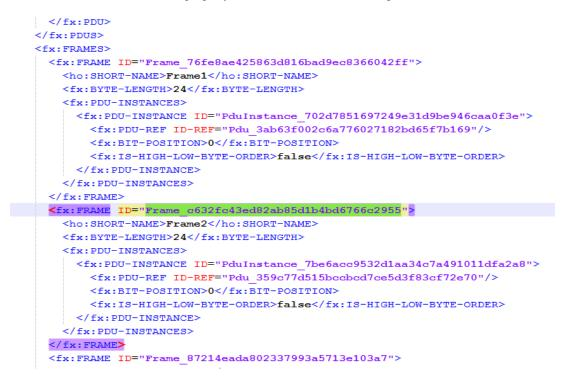
Figure 3-17: A screenshot of a sample frame in a FIBEX file. The highlighted frame is referred in the triggering event described in Figure 3-14 and the unique ID here matches the frame ID-REF in said figure.
