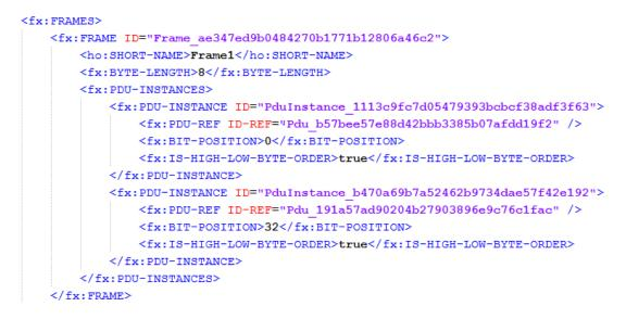
Figure 3-11: A screenshot of a single frame with two PDUs assigned to it in a FIBEX file.
