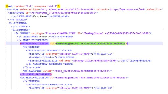
**Figure 3-14**: A screenshot of a single frame triggering event in a complete FIBEX file sample. The frame triggering ID in question is highlighted.
