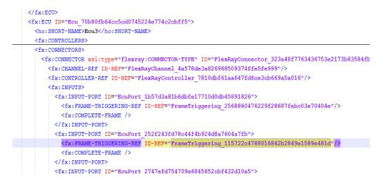
Figure 3-16: A screenshot of the fx:CONNECTORS tab of the ECU receiving the frame sent in Figure 3-14. The highlighted ID-REF matches the unique ID of the frame triggering event given in Figure 3-14.
