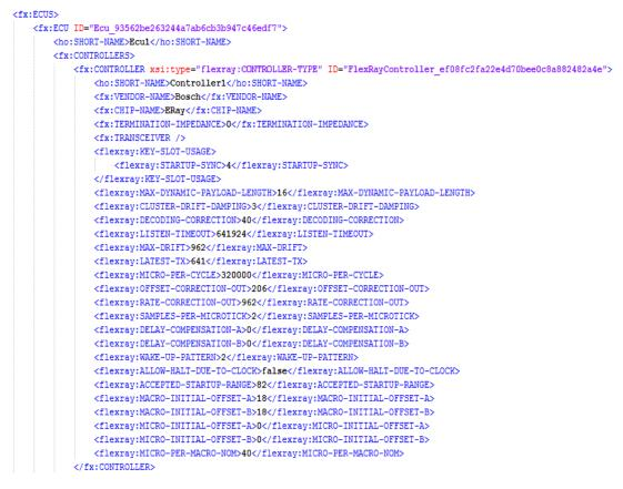
Figure 3-10: A screenshot of the ECU controller parameters as seen in a FIBEX file.
