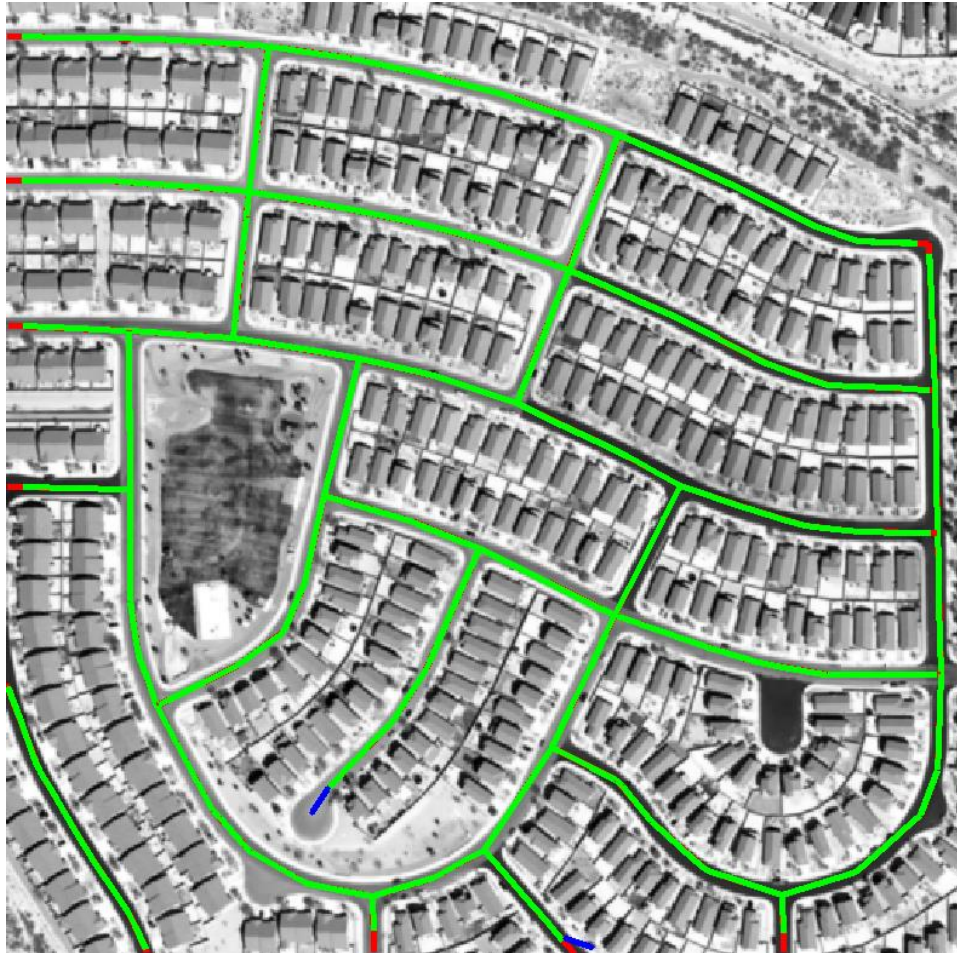
Figure 4-6 Semi-automated system: evaluation results for Test Image 3 (Green – correct extraction, red – missed roads, blue – false extraction).
