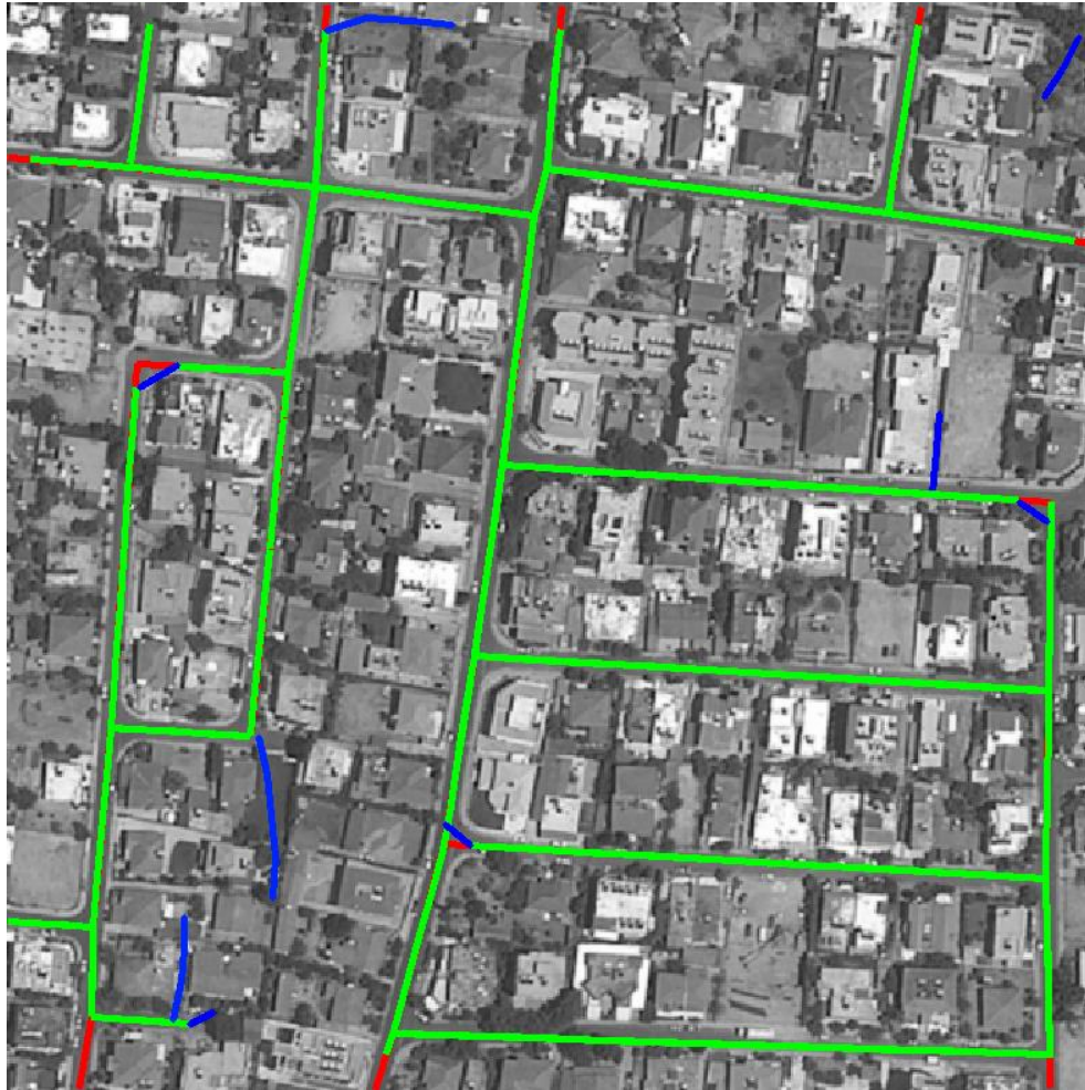
Figure 4-3 Semi-automated system: evaluation results for Test Image 1 (Green – correct extraction, red – missed roads, blue – false extraction).
