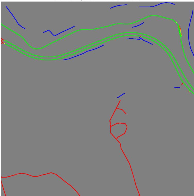
Figure A-6 Evaluation Results for IKONOS Test Image 6: Green – correct extraction, red – missed extraction, blue – false extraction
