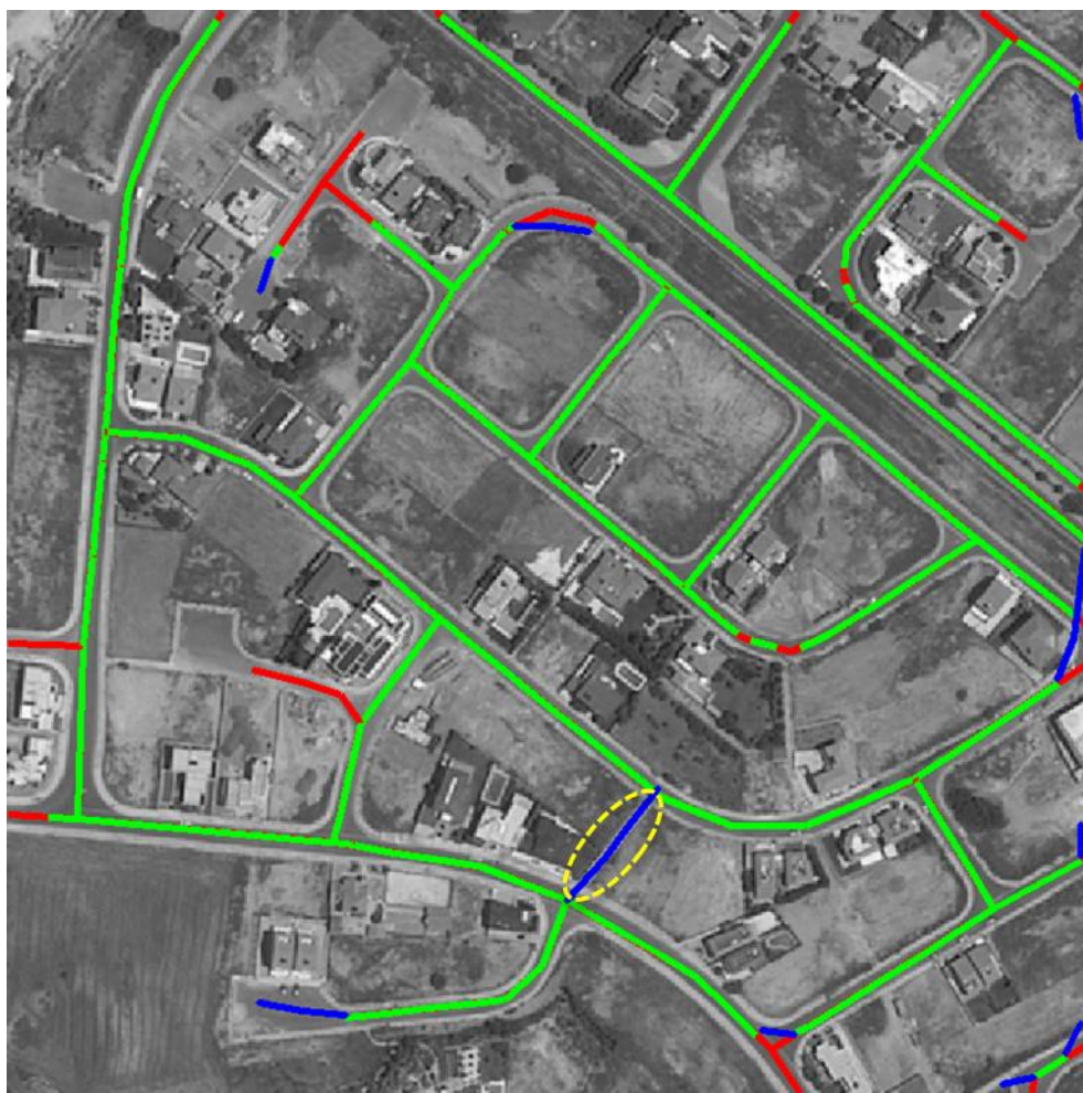
Figure 4-10 Automated system: evaluation results for test image – 2 (Green – correct extraction, red – missed roads, blue – false extraction).
