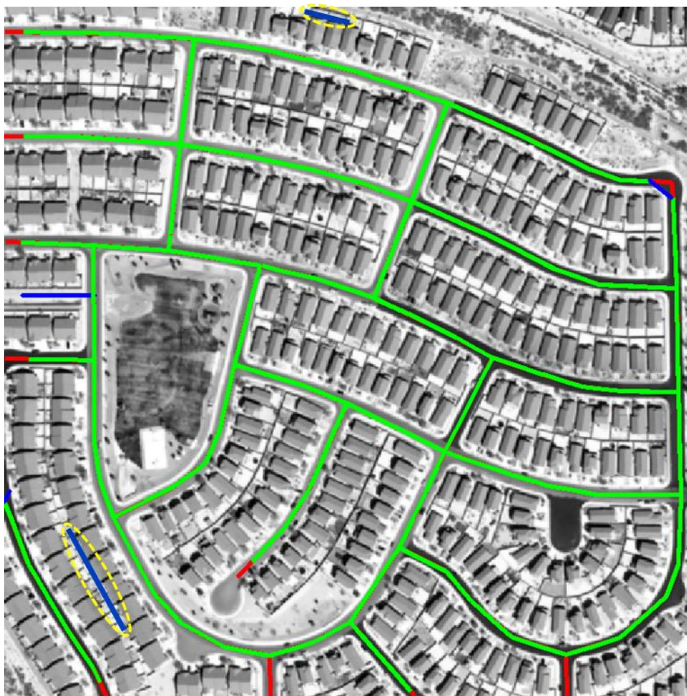
Figure 4-12 Automated system: evaluation results for Test Image 3 (Green – correct extraction, red – missed roads, blue – false extraction).
