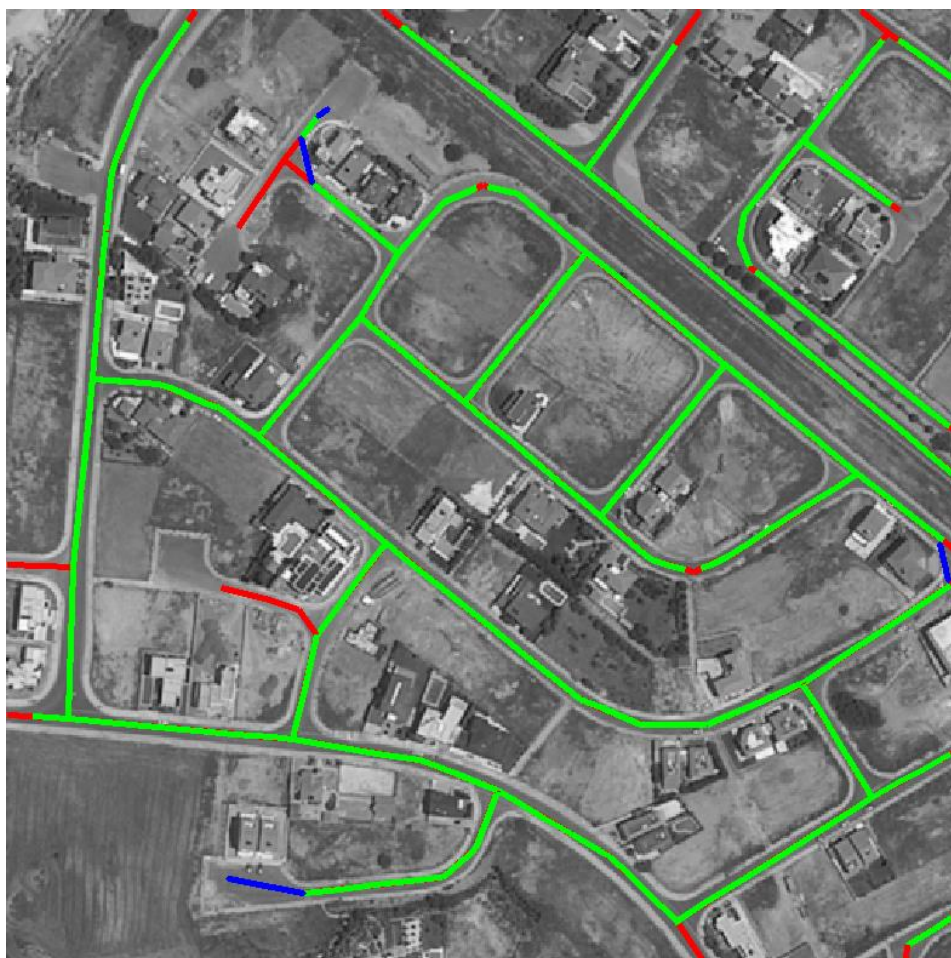
Figure 4-5 Semi-automated system: evaluation results for Test Image 2 (Green – correct extraction, red – missed roads, blue – false extraction).
