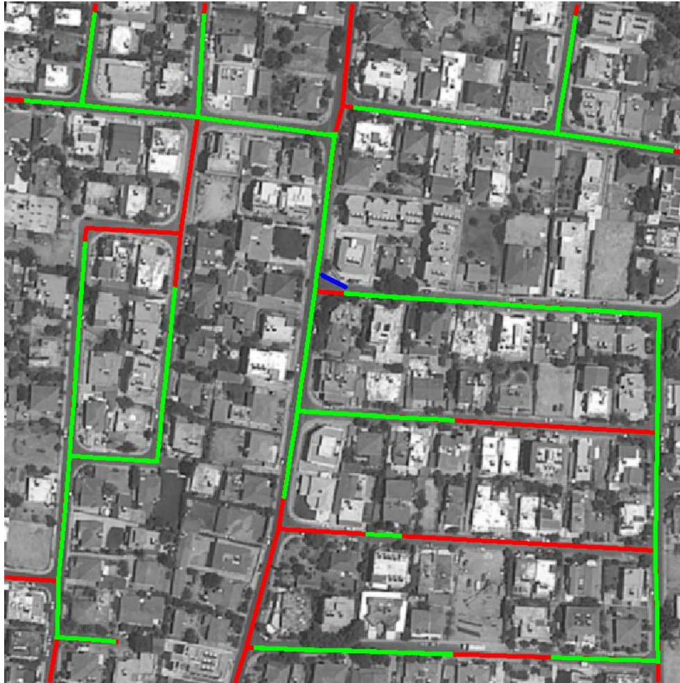
Figure 4-8 Automated system: evaluation results for Test Image 1 (Green – correct extraction, red – missed roads, blue – false extraction).
