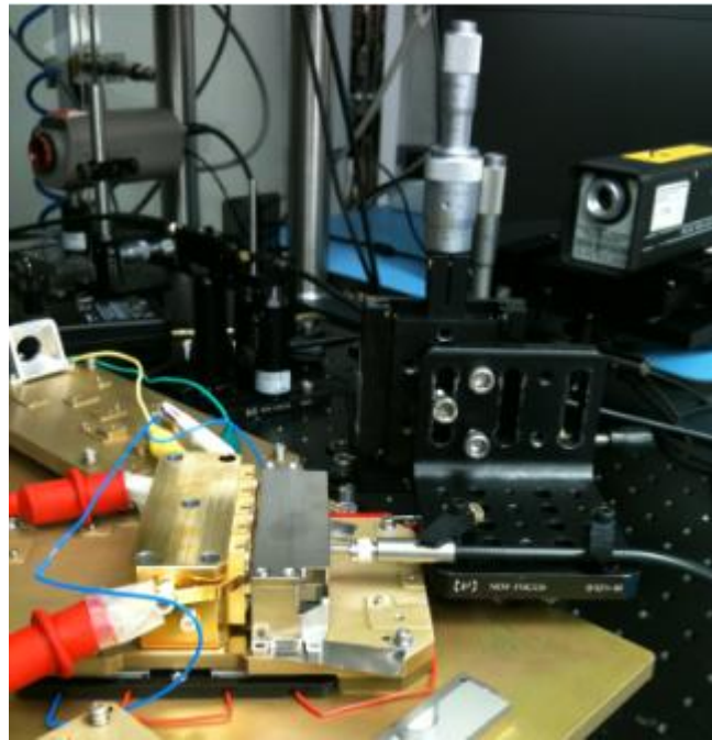
Figure 6.5: The Pump-Beam Uniformity Measurement Setup for the Designed Pump Chamber – Overall View
