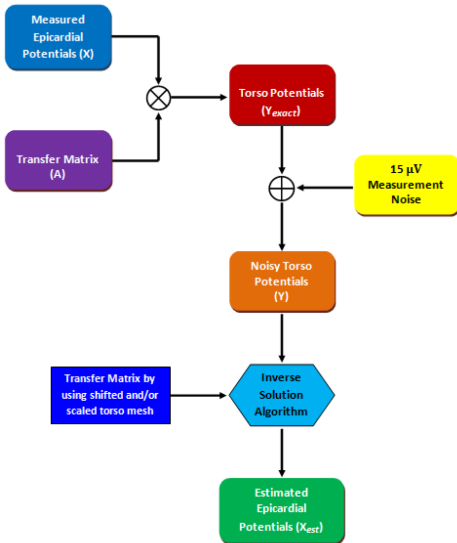
Figure 4.4: The schematic representation of the simulation procedure to study geometric errors
