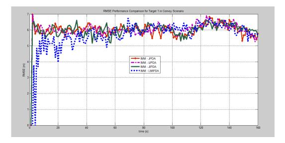
Figure 4.8: RMSE Performance Comparison of IMM-LMIPDA with Optimal Multitarget Tracking Algorithms in Convoy Scenario for Target 1
