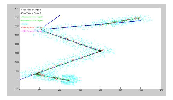
Figure 4.16: Tracking of two targets in clutter where one of the targets stops at initial point
