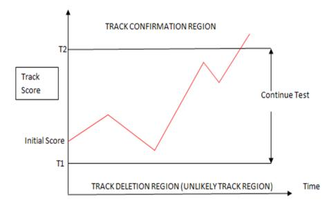
Figure 2.4: Score-Based Track Confirmation and Deletion (Figure is adapted from [10])
