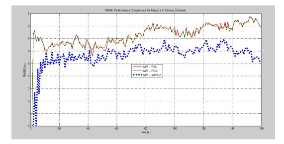
Figure 4.7: RMSE Performance Comparison of IMM-LMIPDA with Single Target Tracking Algorithms in Convoy Scenario for Target 2
