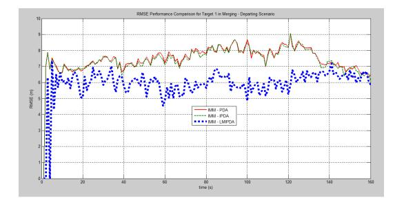
Figure 4.14: RMSE Performance Comparison of IMM-LMIPDA with Single Target Tracking Algorithms in Merging-Departing in junctions Scenario for Target 1
