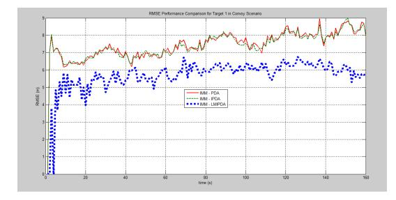
Figure 4.6: RMSE Performance Comparison of IMM-LMIPDA with Single Target Tracking Algorithms in Convoy Scenario for Target 1
