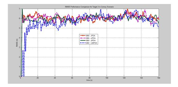
Figure 4.9: RMSE Performance Comparison of IMM-LMIPDA with Optimal Multitarget Tracking Algorithms in Convoy Scenario for Target 2
