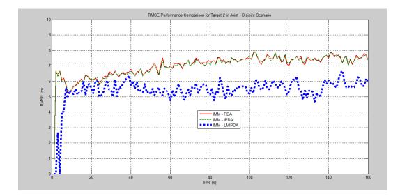
Figure 4.12: RMSE Performance Comparison of IMM-LMIPDA with Single Target Tracking Algorithms in Merging in a junction Scenario for Target 2
