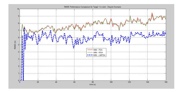
Figure 4.11: RMSE Performance Comparison of IMM-LMIPDA with Single Target Tracking Algorithms in Merging in a junction Scenario for Target 1
