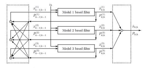
Figure 2.2: Structure of the IMM Estimator (with three models) (Figure is adapted from [4])
