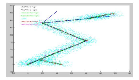
Figure 4.10: Tracking of two targets in clutter merging in a junction
