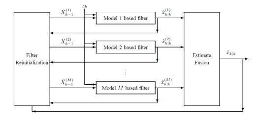
Figure 2.1: Structure of a Recursive MM Estimator (Figure is adapted from [4])
