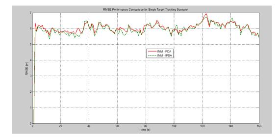
Figure 4.2: RMSE Performance Comparison of IMM-PDA with IMM-IPDA in Single Target Tracking Scenario
