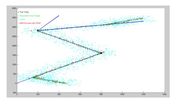
Figure 4.1: Tracking of single target in clutter
