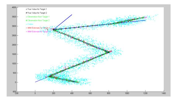
Figure 4.3: Tracking of two targets in clutter moving in a convoy fashion
