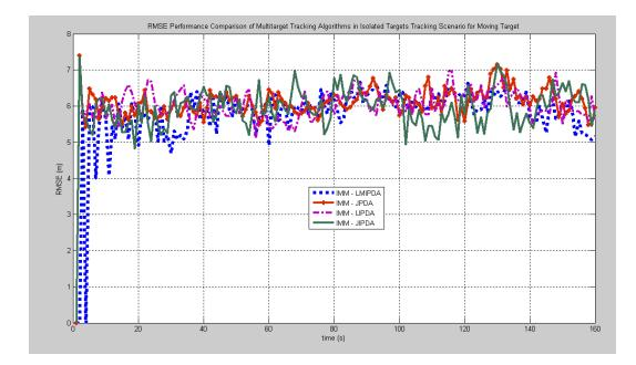
Figure 4.17: RMSE Performance Comparison of Multitarget Tracking Algorithms in Single Target (Isolated Targets) Tracking Scenario for Moving Target
