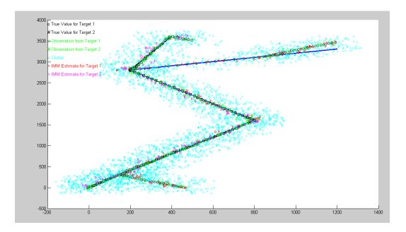
Figure 4.13: Tracking of two targets in clutter merging-departing in junctions
