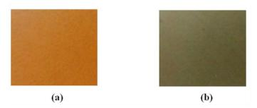
**Figure 3.14:** CHO /  $Ph_2I^+PF_6^-$  / PS2 mixture (a) before exposure to solar irradiation, and (b) after 5 minutes of exposure.
