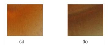
**Figure 3.13:** CHO /  $Ph_2I^+PF_6^-$  / PS1 mixture (a) before exposure to solar irradiation, and (b) after 5 minutes of exposure.
