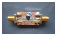
Figure 4.1: Fixture for testing the transistors before mounting on the main board.
