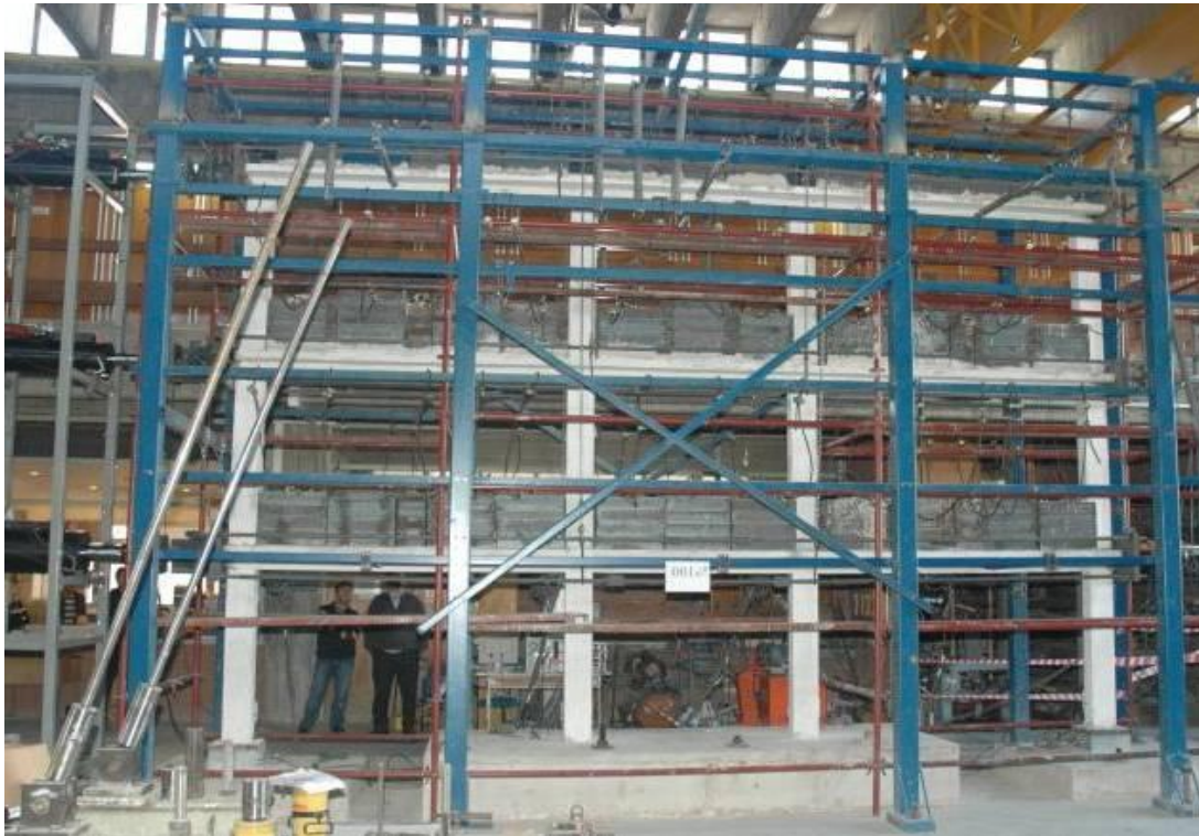
Figure 2. 4 Test specimen and pseudo-dynamic testing system scheme
