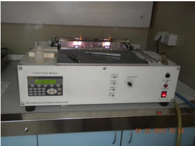
Figure 3.1. Bead Fusion Machine
