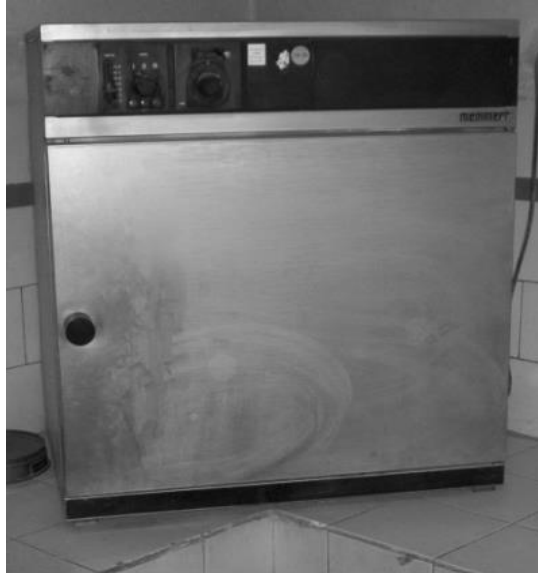
Figure 3.3. Oven used to dry the materials
