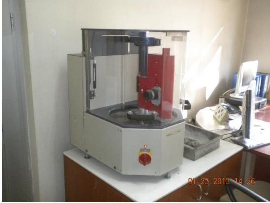
Figure 3.10. Automatic Vicat Device
