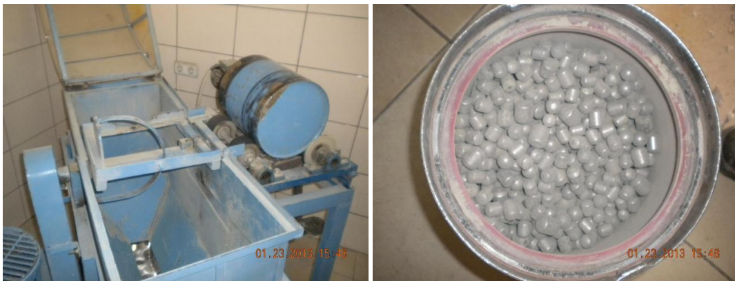
Figure 3.5. Laboratory mill and charge
