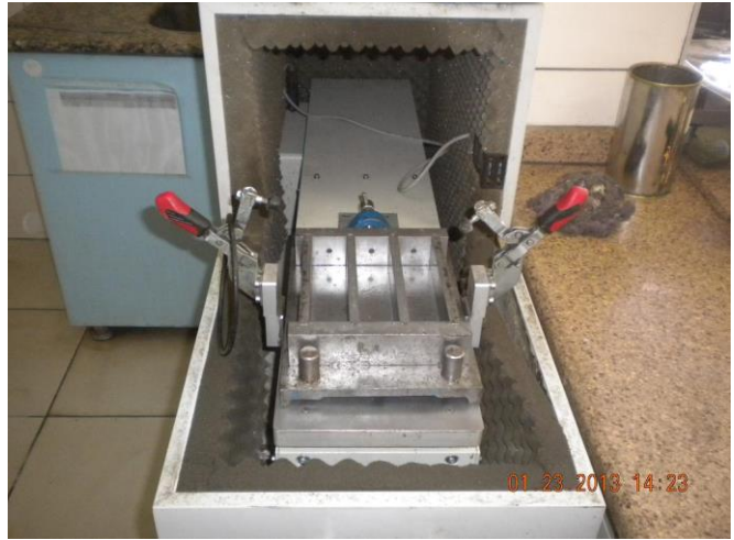
Figure 3.7. Prism sample mold and vibration shock table
