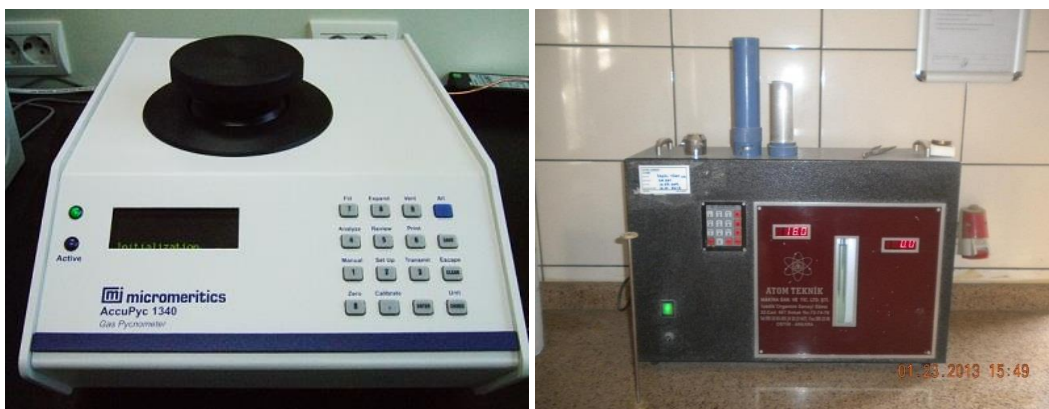
Figure 3.6. Gas Pycnometer and Blaine fineness Apparatus
