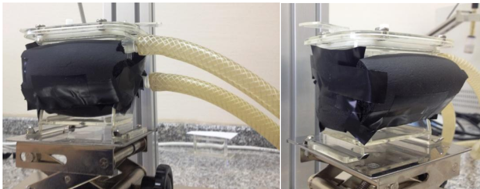
Figure 33. Insulated water jacket of the measurement unit
