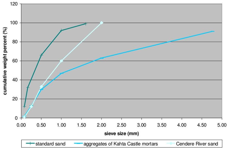
Figure 2.1 Particle size distribution of standard sand and Cendere River sand used in the preparation of repair mortar mixtures.
