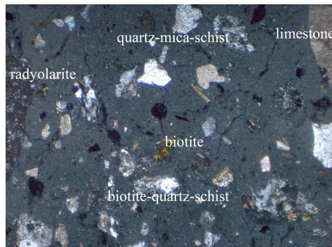
Figure 3.16 Thin section view showing the aggregates used for the preparation of pozzolanic mortars (cross nicols 2.5x).
