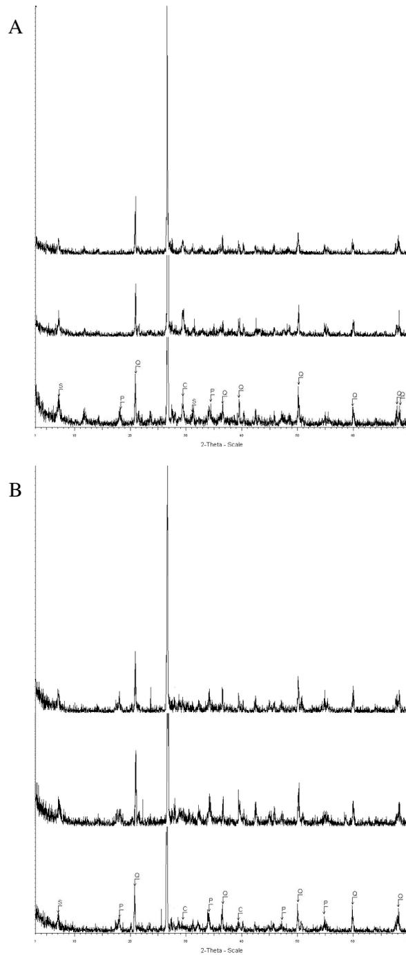
Figure 3.23 XRD traces of the mortar set RM-MS-X after 28, 30 and 90 days (from bottom to top) of curing time (A external surface, B internal surface below). C: Calcite, Q: Quartz, P: Portlandite
