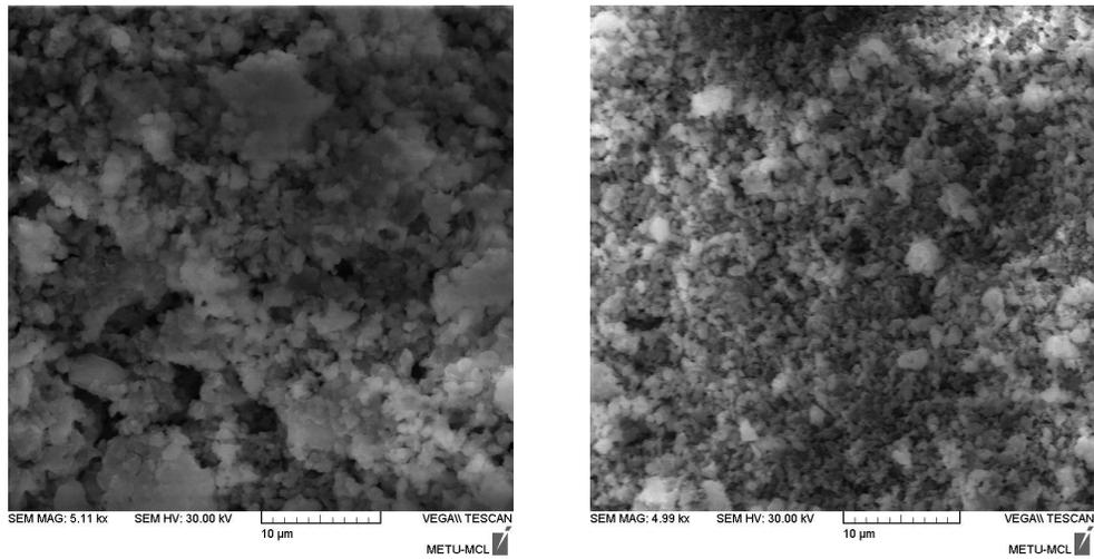
Figure 3.17 SEM image of binder matrix of mortar sample from Kahta Castle (left). White lump in the mortar matrix (right) showing the distinction between the particle sizes of the crystal aggregates in the binder matrix and the white lump.
