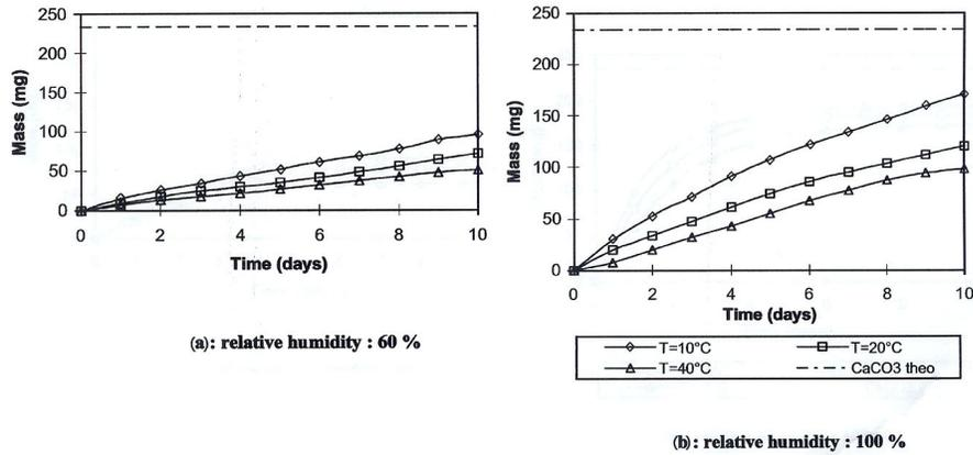
Figure. 1.1 Effect of relative humidity on carbonation of  $\text{Ca(OH)}_2$  in dry powder form. Y axis shows the weight increase of 661 mg dry  $\text{Ca(OH)}_2$  due to carbonation through ten days (Dheilly et al. 2002).
