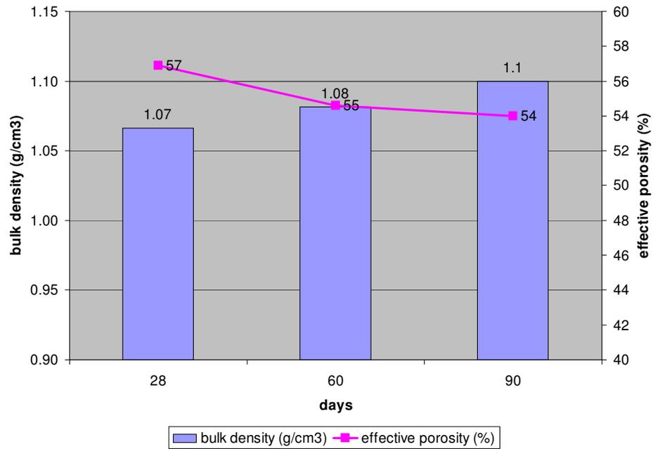
Figure 3.3 Bulk density and porosity change in repair mortars, RM-MC-Z at 28, 60 and 90 days in the laboratory.
