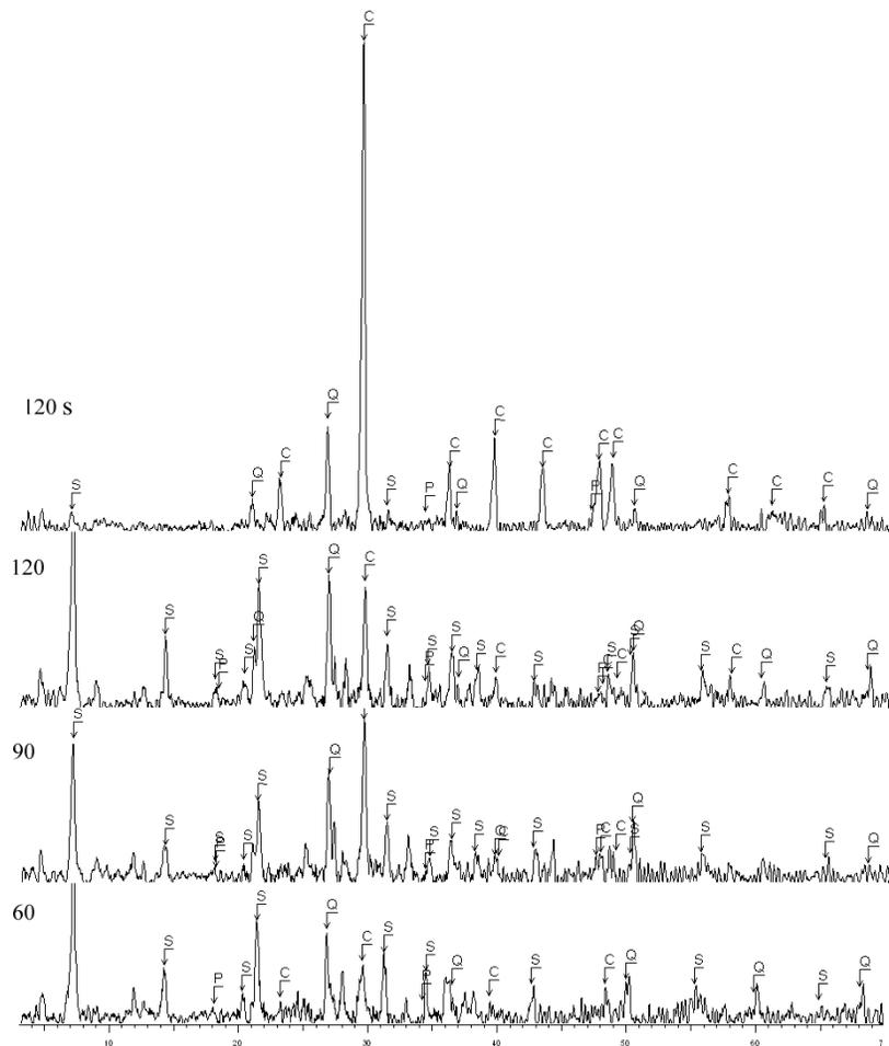
Figure 3.26 XRD traces of the mortar cubes RM-MC-Y (external surface) at 60, 90 and 120 days (from bottom to top) of curing time. 120 s denotes the XRD trace of mortar cube left on site for 120 days. C: Calcite, Q: Quartz, P: Portlandite, S: Stratlingite
