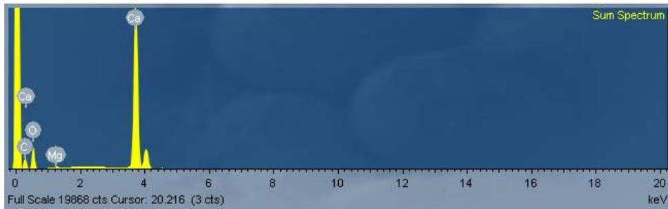
Figure 3.18 EDX analyses of the white lump in Kahta Castle mortars.
