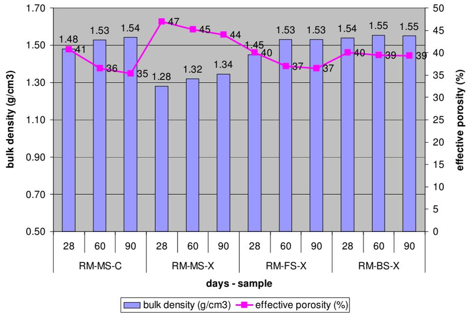
Figure 3.1 Bulk density and porosity of the repair mortars, RM-MS-X, RM-FS-X, RM-BS-X and control, RM-NS-C.
