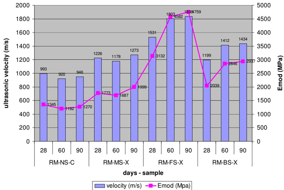
Figure 3.7 Ultrasonic velocity and modulus of elasticity values of repair mortars (RM-MS-X, RM-FS-X, RM-BS-X and control (RM-NS-C)).
