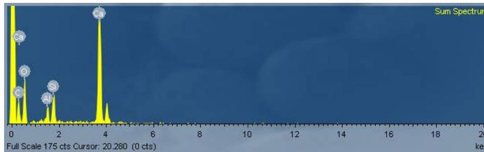
Figure 3.20 EDX analyses of needle like CASH structure.
