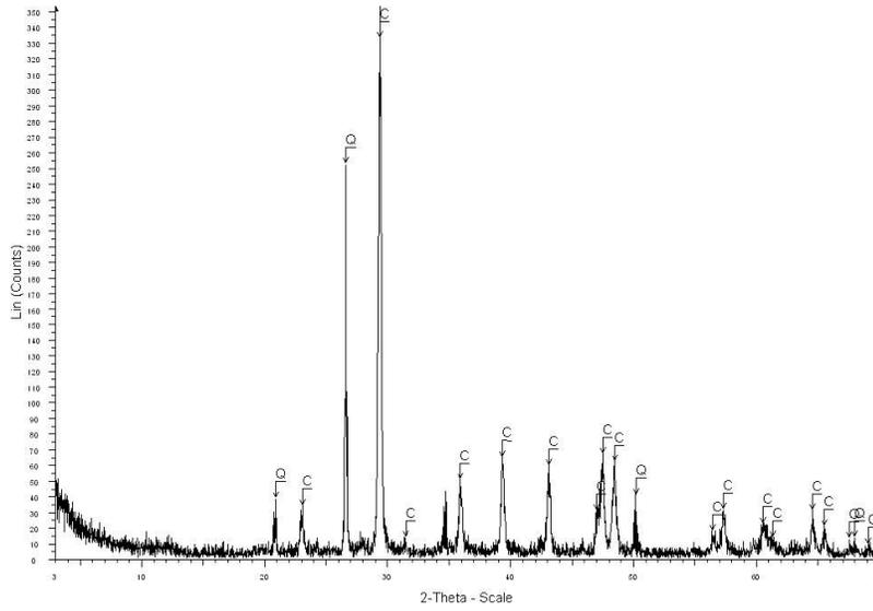
Figure 3.21 XRD traces of a mortar sample from Kahta Castle. C: Calcite, Q: Quartz
