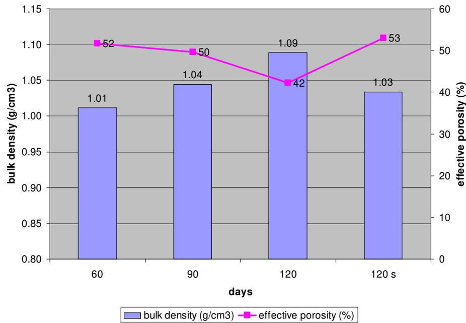
Figure 3.2 Bulk density and porosity change in repair mortars, RM-MC-Y at 60<sup>th</sup>, 90<sup>th</sup> and 120<sup>th</sup> days in the laboratory. (120 s: denotes the mortars left on site at Nemrut Dağ Monument for 120 days.)
