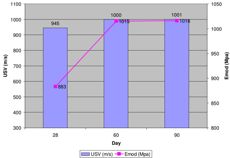
Figure 3.9 Ultrasonic velocity and modulus of elasticity values of prepared pozzolanic lime mortars, RM-MC-Z from day 28 to day 90.
