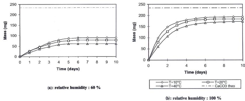
Figure 1.2 Weight increase of dry powder  $\text{Ca(OH)}_2$  through ten days in a  $\text{CO}_2$  rich atmosphere (Dheilly et al. 2002).
