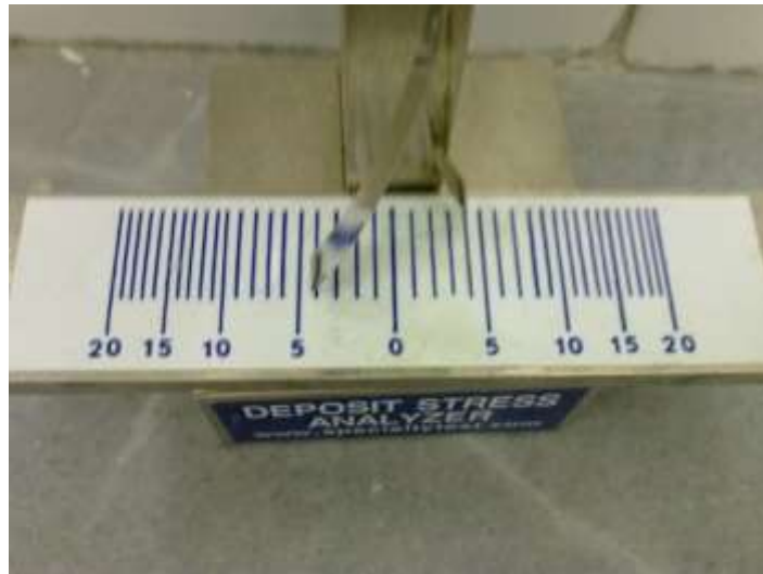
Figure 4.14 Deposit stress analyzer showing number of increments, U, in run 11.
