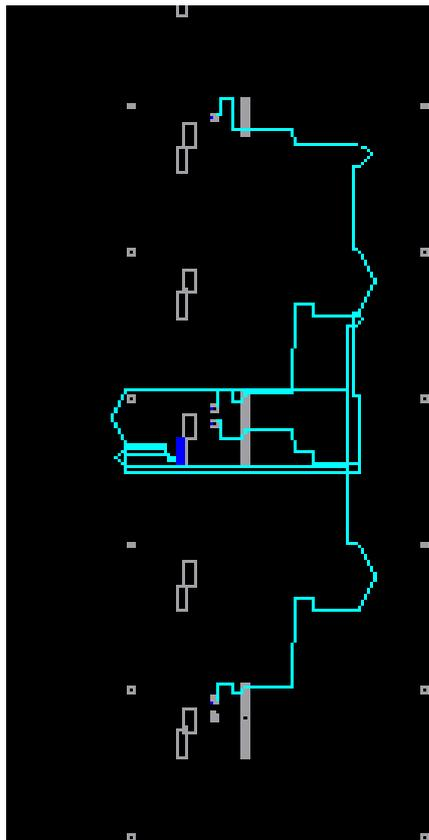
Figure 5.12: Placed and routed 2-to-1 MUX
