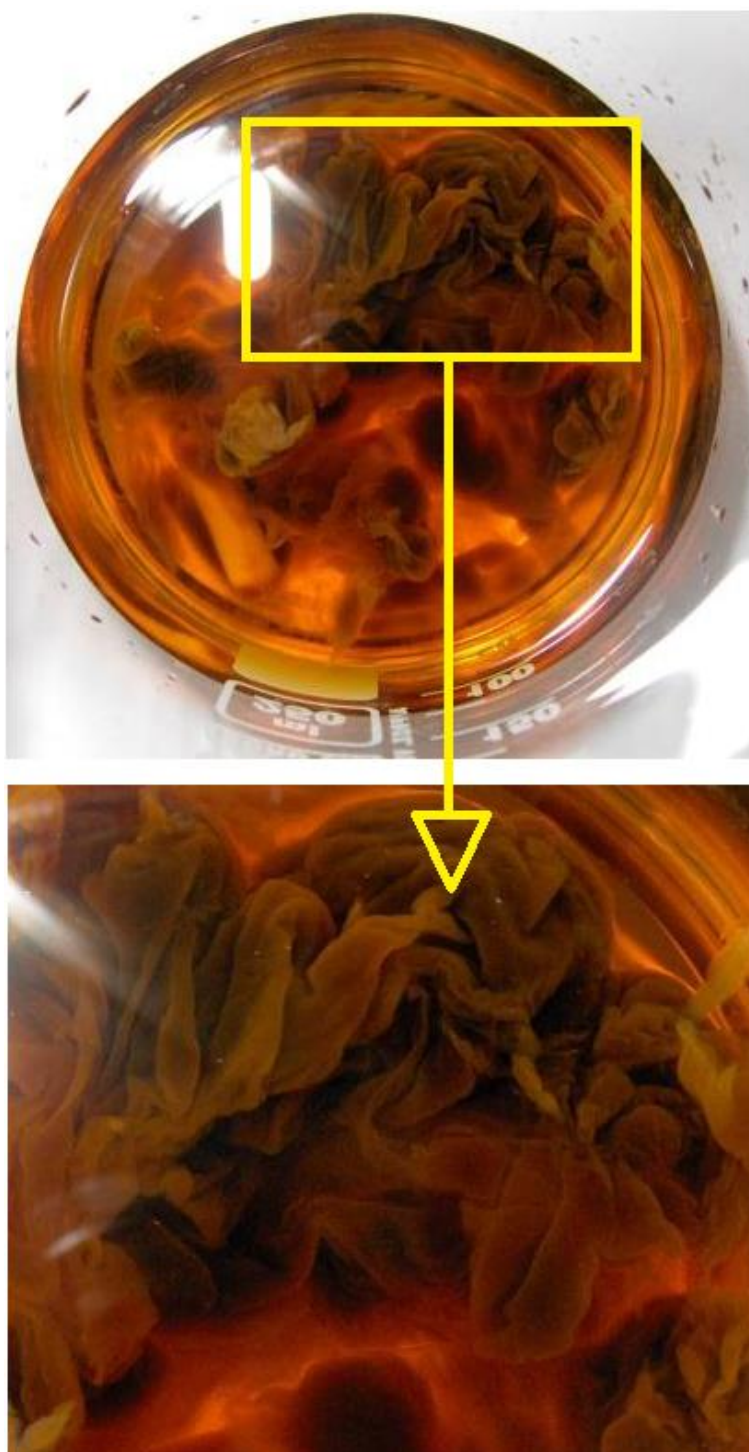
Figure 1.3. Picture of regenerated cellulose right after its precipitation by the addition of water to the ionic liquid cellulose solution (Haykir, 2013).
