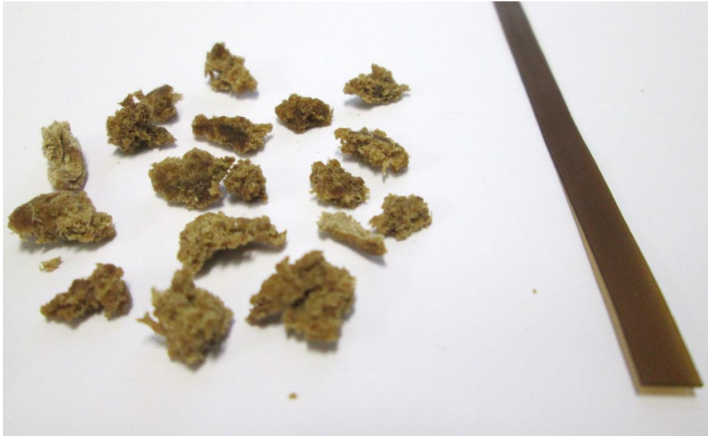
Figure 7.1. Appearance of hemicelluloses extracted from corn cobs prior to being fed to the extruder (left) together with a hemicellulose strip produced from these polymers via extrusion (right).
