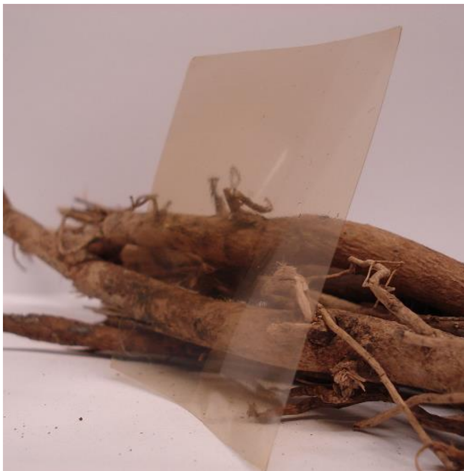
Figure 1.6. A hemicellulose based polymeric film pictured in front of the cotton stalks it was obtained from.
