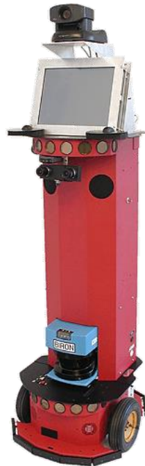
Figure 2.2- BIRON has a Sony EVID31 pan-tilt color camera on the top. [7]
