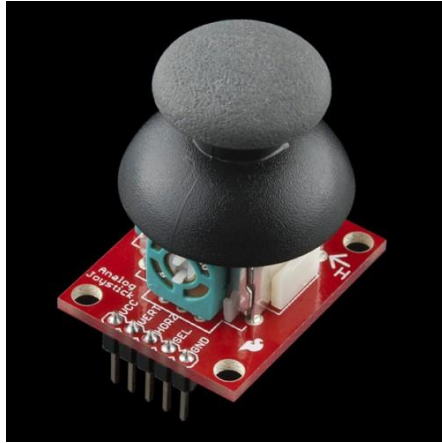
Figure 3.1-Joystick for controlling zoom in and out of HDR-TD30V
