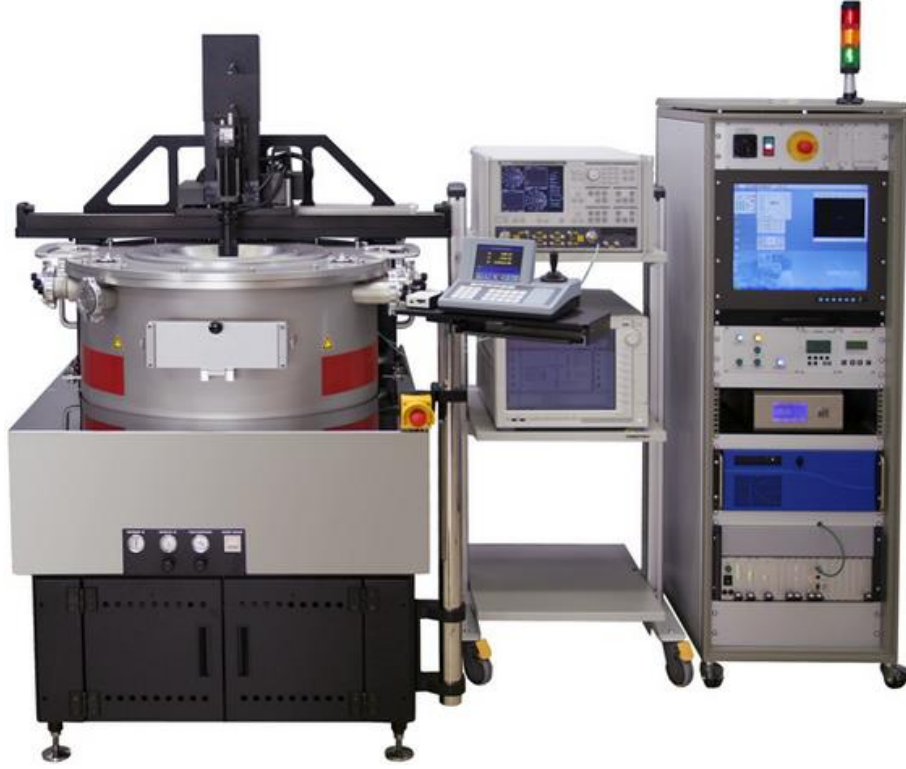
Figure 4.1. The photograph of SÜSS MicroTec PAV 200 equipment utilized in the thermal conductance, responsivity, and absorptance measurements.
