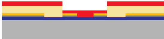
(b) Sol-gel VO x deposition and heat treatment at 120°C for physical water removal.
