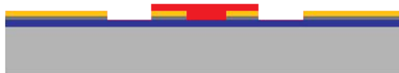
(c) Stripping the photoresist in acetone which also lifts off the VO x layer residing on top of it.
