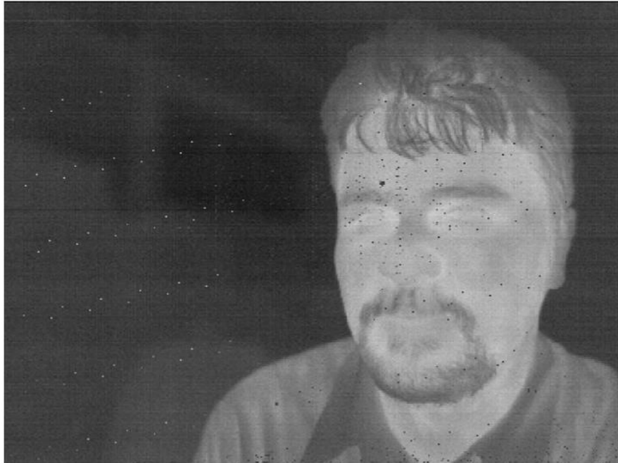
Figure 1.10. An image obtained by 35 \mu\text{m} pixel 384x288 microbolometer FPA fabricated at METU MEMS Center [18].
