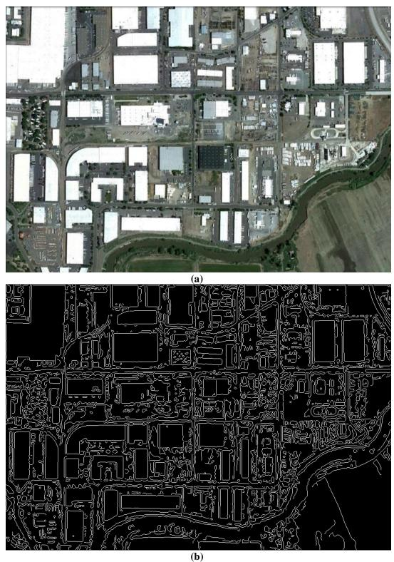
(b) Figure 47 (a) A satellite image of an industrial zone taken from Google Earth, (b) its edge map and rectangle detections using (c) WHT in CC and (d) RDDI.
