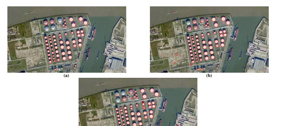
(c) Figure 71 Recognized POLs on the image in Figure 66 using (a) MHT, (b) MHT CC and (c) RCD CC.
