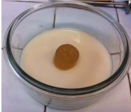
Figure 6-6: Phantom-1 before the second fat layer is poured.
