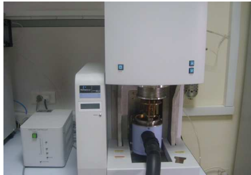
Figure 5-5: Perkin Elmer Pyris Diamond Dynamic Measurement Analyzer (DMA) in METU Central Laboratory.
