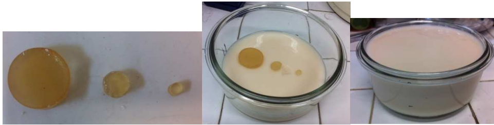
Figure 5-7: Homogeneous breast phantom including 3 different size tumor phantoms at 30 mm depth. Left: Tumor phantoms used in the breast phantom, Middle: Tumor phantoms placed on the fat phantom at the first stage. Right: Final condition of the breast phantom after the second stage.
