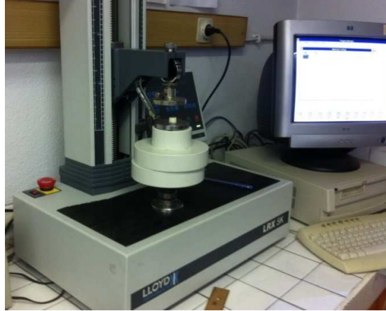
Figure 5-6: Lloyd LRX 5K materials testing machine in METU BIOMATEN laboratory testing fat phantom sample. The stress-strain relationships of the different phantom types are measured using a 100 N load cell. The samples were 15 mm in diameter and 10 mm in height.
