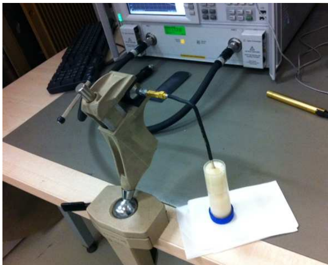
Figure 5-2: Dielectric measurement of the breast fat phantom using network analyzer.
