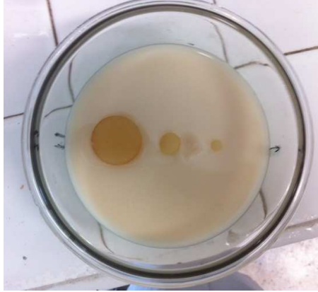
Figure 6-21: Phantom-2 before the second fat layer is poured.
