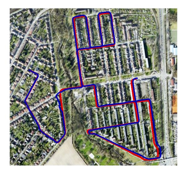
Figure 4.6: 2D Trajectory plotted on Google Earth data - Ground Truth (blue) vs Hybrid Stereo-VO/IMU (red).
