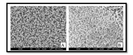
**Figure 1.3** SEM images of ZnO nanorods grown on glass substrates coated with gold (**A**) The ZnO nanorods only and (**B**) ZnO nanorods with immobilized GAO enzyme (Khun *et al*, 2012).
