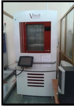
Figure 4.6 Air conditioning cabin
