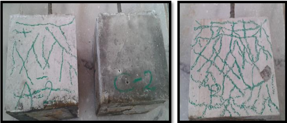
Figure 5.8 Cube specimens for pullout strength of G-A, G-C, and G-B concretes, respectively
