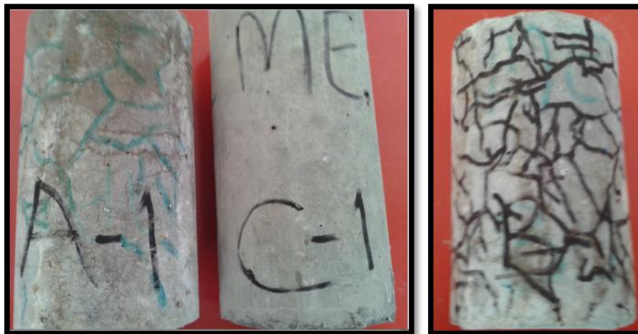
Figure 5.7 Cylindrical specimens for modulus of elasticity of G-A, G-C, and G-B concretes, respectively
