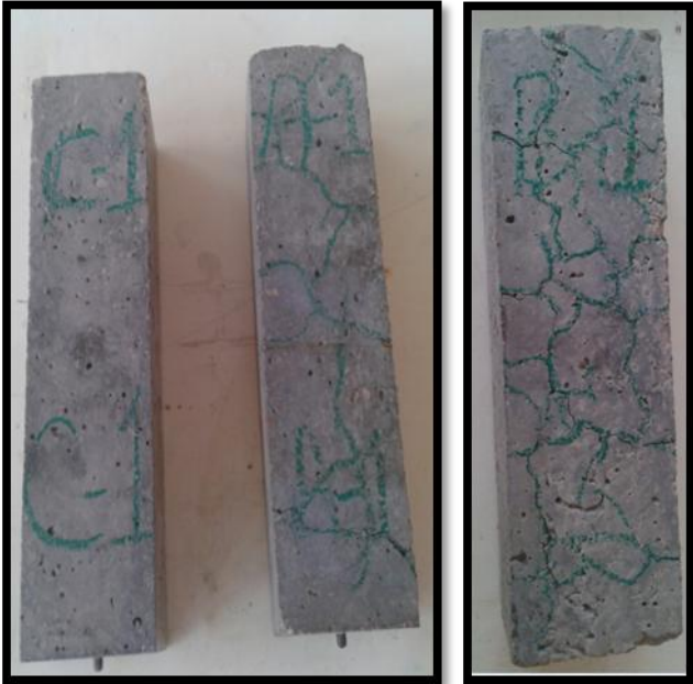
Figure 5.5 Prismatic specimens of G-C, G-A, and G-B concretes respectively
