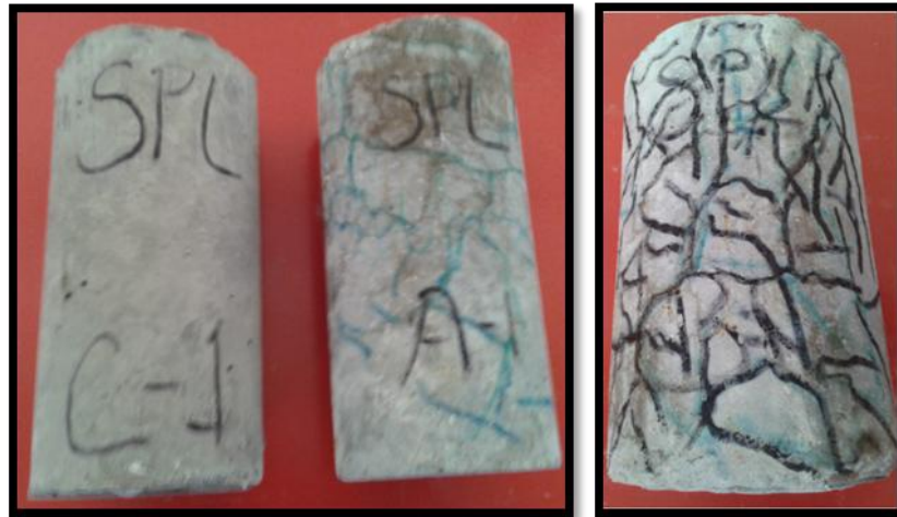
Figure 5.6 Cylindrical specimens for tensile splitting strength of G-C, G-A, and G-B concretes, respectively
