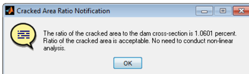
Figure 2.37 Message window which shows the ratio of the cracked area to the dam cross section
