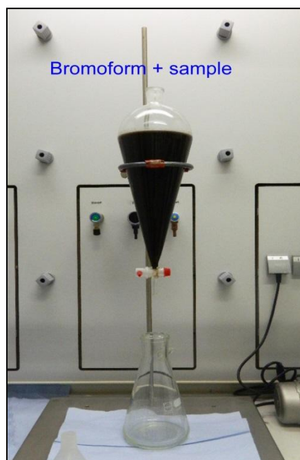
Figure A.2 The heavy liquid bromoform and sample are mixed in a glass; then wait for sometime until the heavier and heaviest minerals are separated according to their relative density with respect to the density of the liquid. Then the mixture is run through separating funnel.
