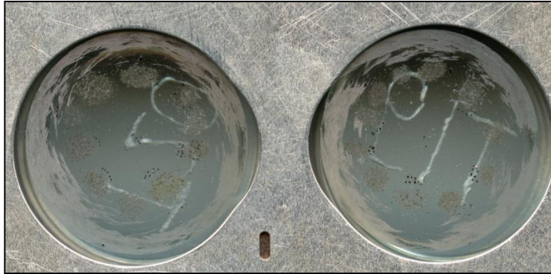
Figure A.5 View of mounted and polished zircon grains ready for cathodoluminescence imaging.
