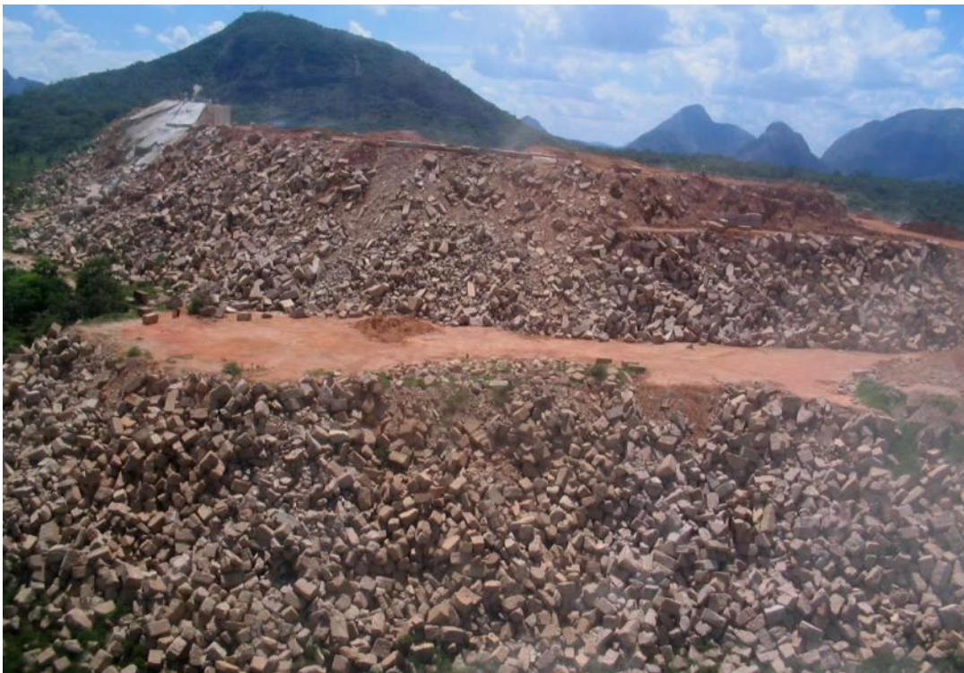
Figure 1 Rock fragments deriving by cutting and sawing of stone [13]
