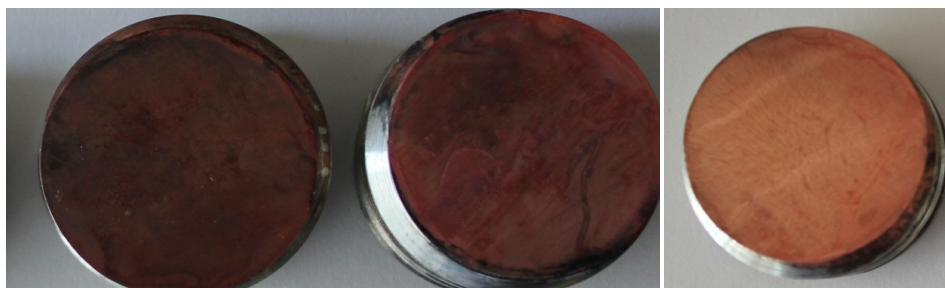
Figure 4.33 Depositions before and after changing zincate solution.
