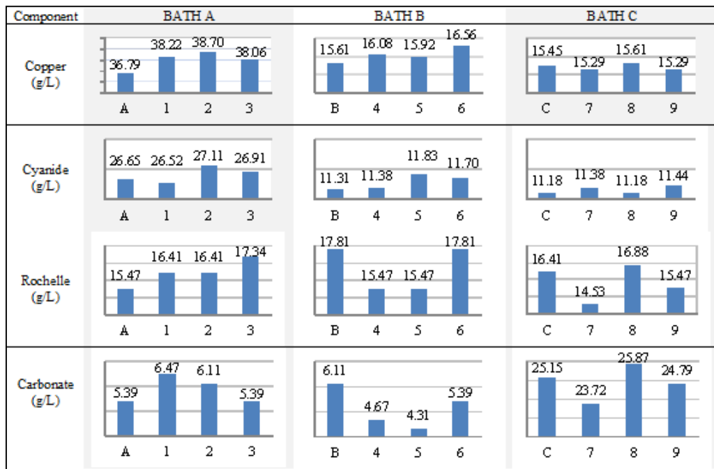
Figure 4.17 The changes in copper, cyanide, Rochelle and carbonate concentrations.
