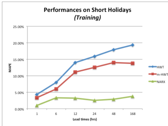
Figure 51. Training performances of three models on short holidays for different forecast horizons in Noord data set.
