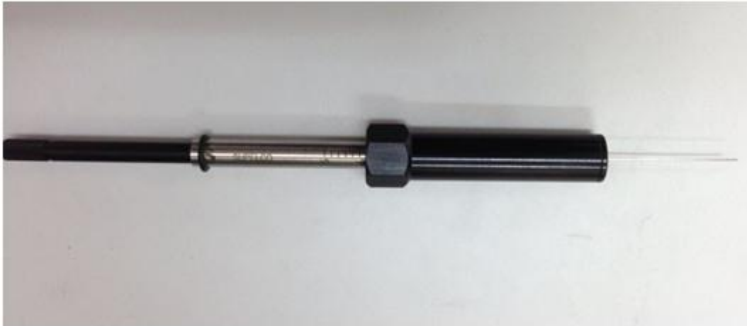
Figure 2.3 SPME device with microfiber used for GC injection.
