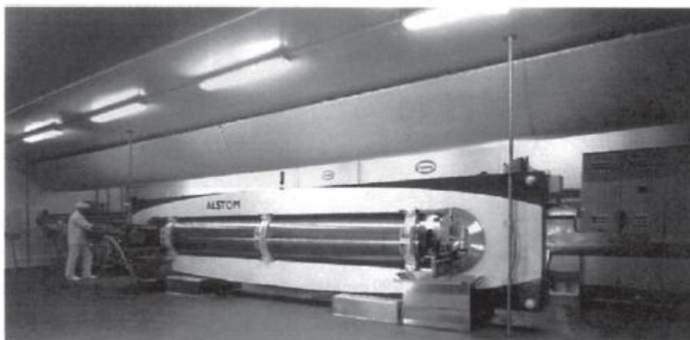
Figure 1.5 Industrial HHP System for ham processing in Spain (Martin, Barbosa-Cánovas, & Swanson, 2004).
