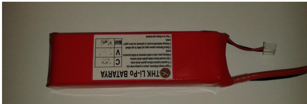
Figure 4-4: Li-Po Battery used in the Robot
