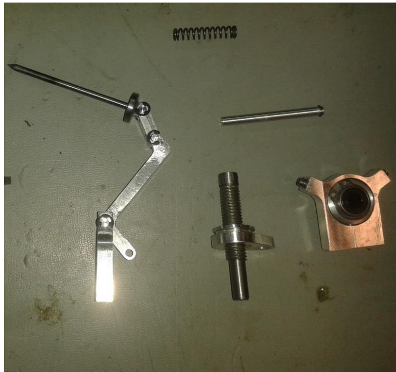
Figure 3-28: Components of the Manufactured Piercing Mechanism
