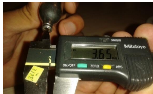
Figure 3-14: Measurement of the Maximum Possible Orifice Area of the 12g CO2 cartridge
