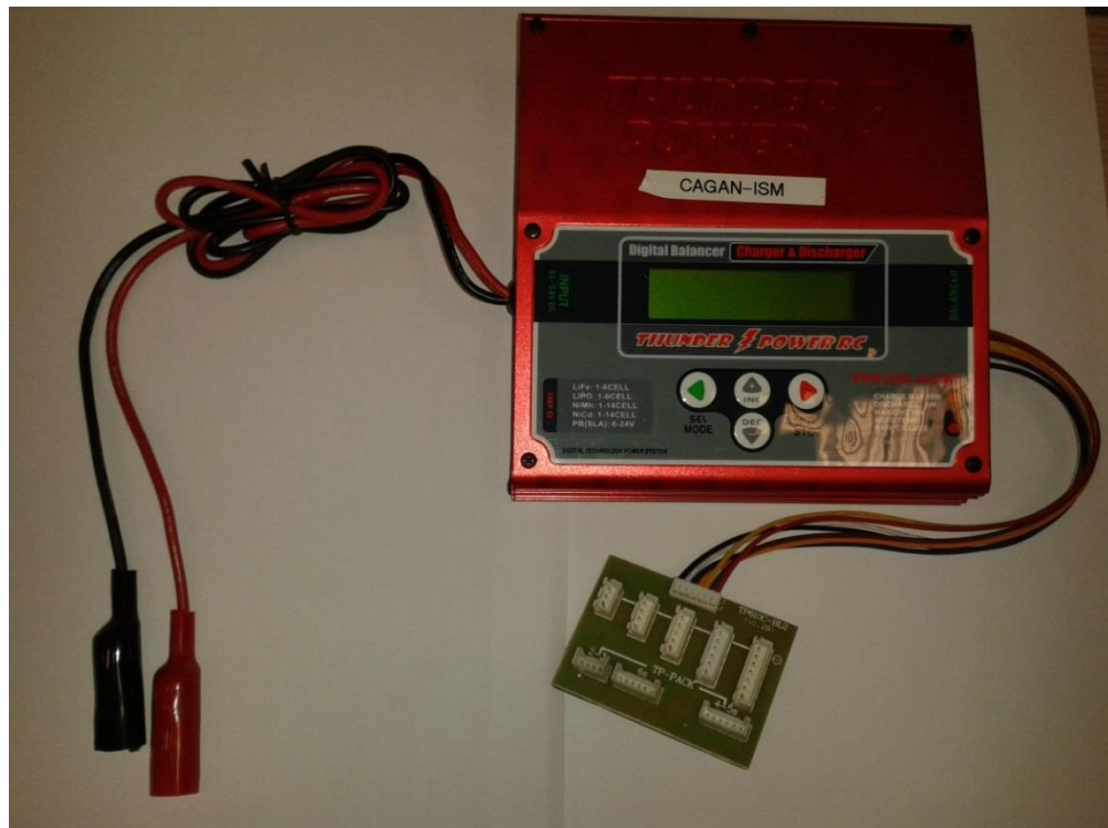
Figure 4-5: Balanced Battery Charger
