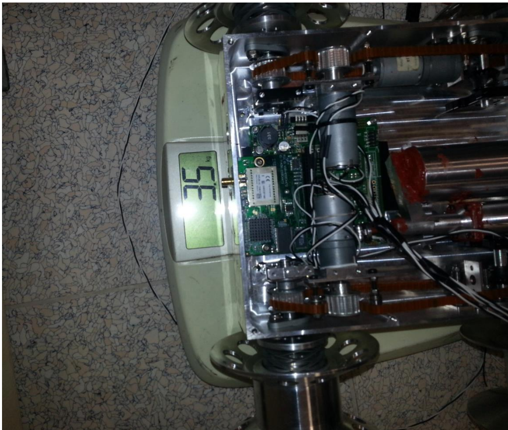
Figure 3-34: Measurement of the Weight of the Robot
