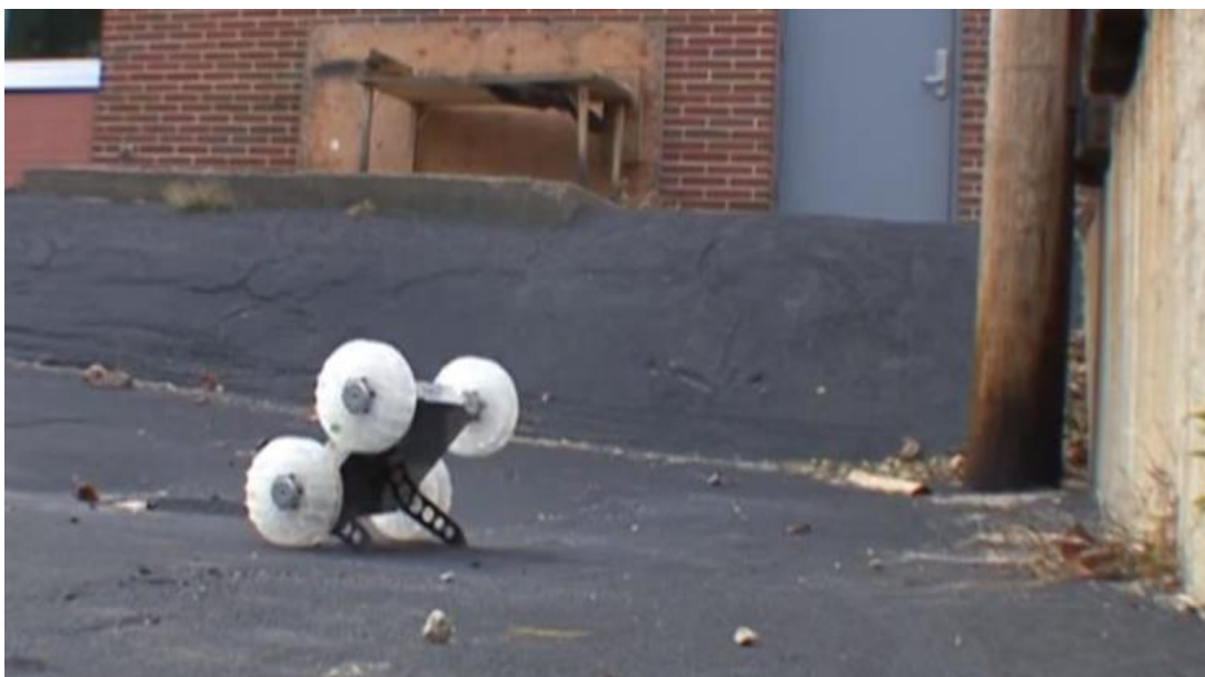
Figure 1-7: Sand Flea Positioning Itself Before A Jump
