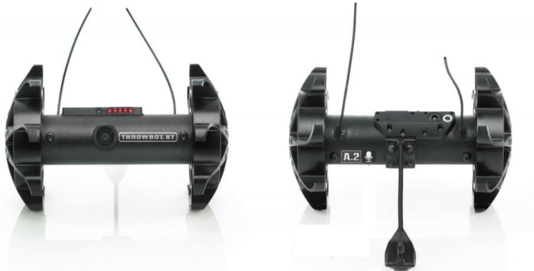
Figure 1-4: Recon Robotics Scout XT Throwable Robot
