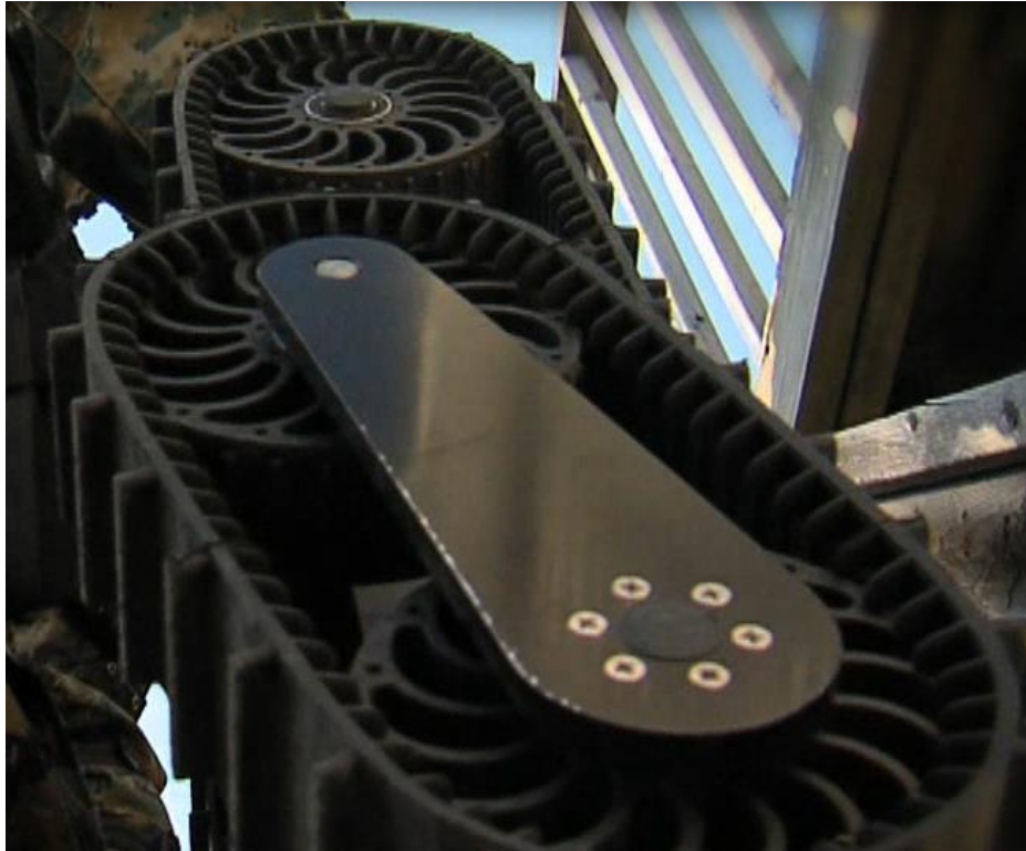
Figure 2-1: Resilience in wheel is achieved through curved arches in this iRobot Negotiator
