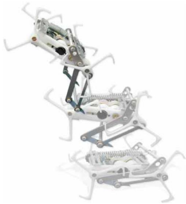
Figure 1-9: MiniWhegs Robot during its Jump
