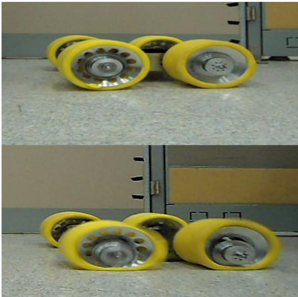
Figure 2-10: Cone Wheel shown in natural state in top and deflected state on bottom
