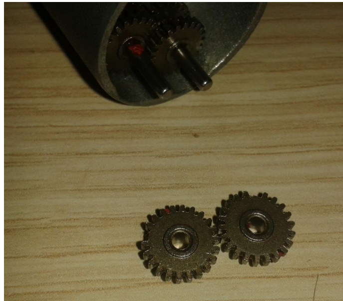
Figure 3-36: Fractured Gears of the Left Tilt Motor's Gearbox
