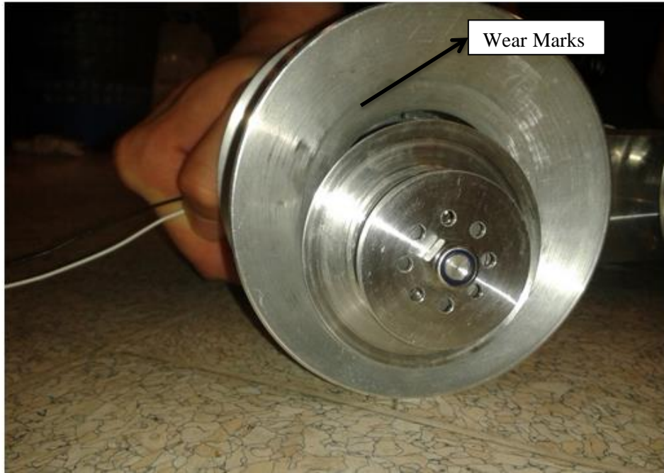
Figure 2-11: Marks of wear on the cone wheel
