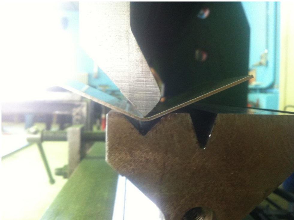
Figure A.6 1.5-mm-thick steel fully loaded stage
