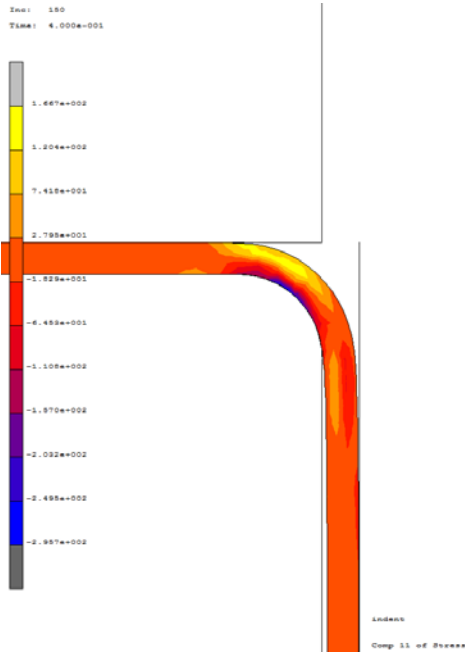
Figure 5.18 Normal stress distribution in longitudinal direction in steel 1 for 1.5-mm-thick sheet with 4 mm die radius at the fully loaded stage
