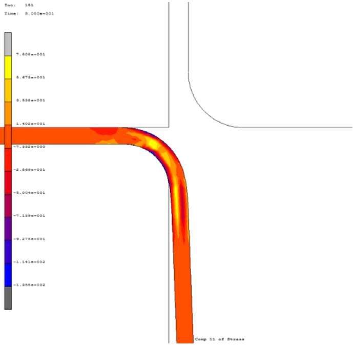
Figure 5.19 Residual normal stress distribution in longitudinal direction in steel 1 for 1.5-mm-thick sheet with 4 mm die radius at the unloaded stage
