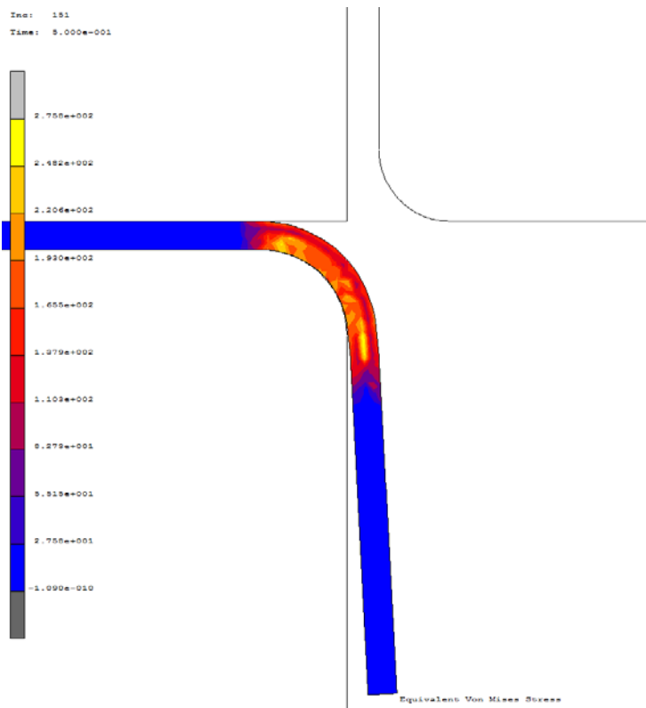
Figure 5.17 Residual von Mises stress distribution in steel 4 for 2-mm-thick sheet with 6 mm die radius at unloaded stage
