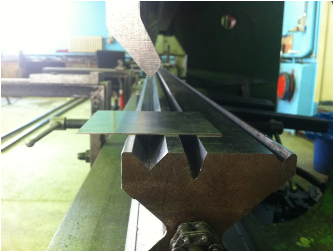
Figure A.4 1-mm-thick steel just before operation
