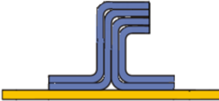
Figure 18. Symmetric modeling configuration of the J-type stiffener
