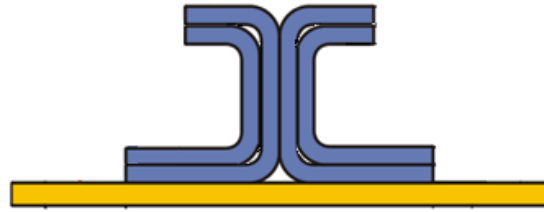
Figure 23. Symmetric modeling configuration of the T-type stiffener
