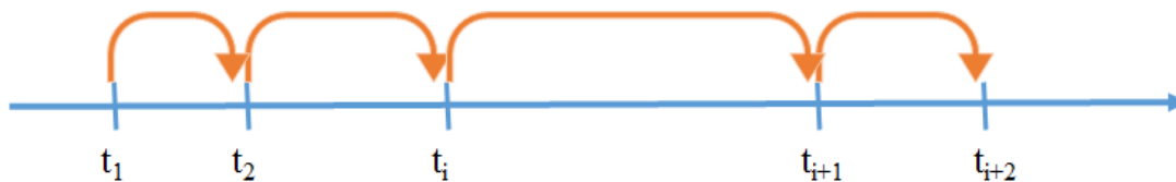
Figure 2.1 : Principle of Discrete Event Simulation (Adapted from [4])
