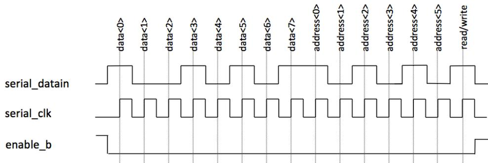
Figure 4.22: Serial interface timing diagram
