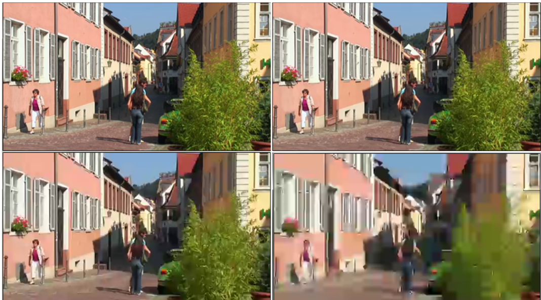
Figure 3.7: Variation in the Image Quality by QP values of (Top-left) 16, (Top-right) 24, (Bottom-left) 36, and (Bottom-right) 48.
