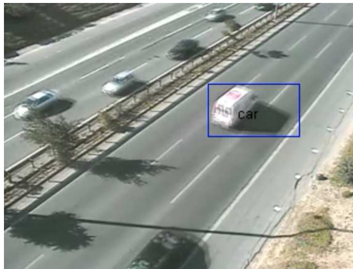
Figure 4.13. An example of incorrect classification when only blob feature used
