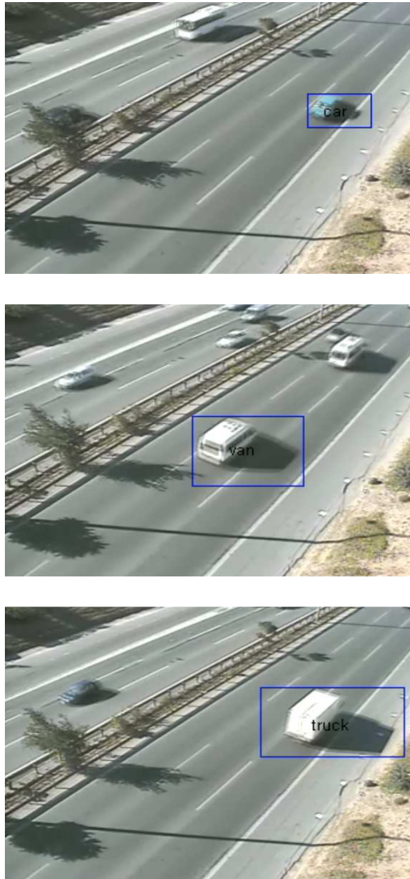
Figure 4.6. Examples of correct classification of the vehicles on Video-2
