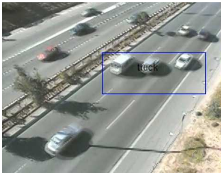
Figure 4.10. Misclassification due to the shadow
