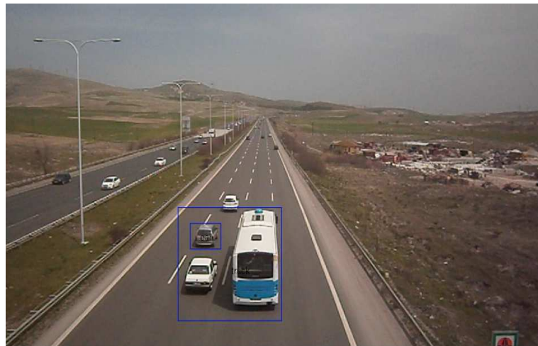
Figure 4.18. Misclassification due to the shadow
