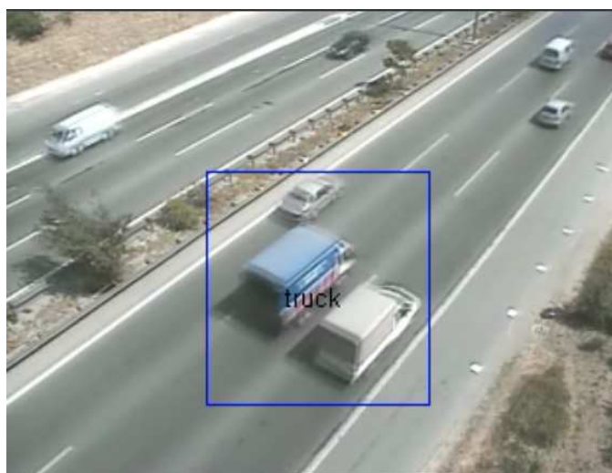
Figure 4.8. Misclassification due to the perspective occlusion
