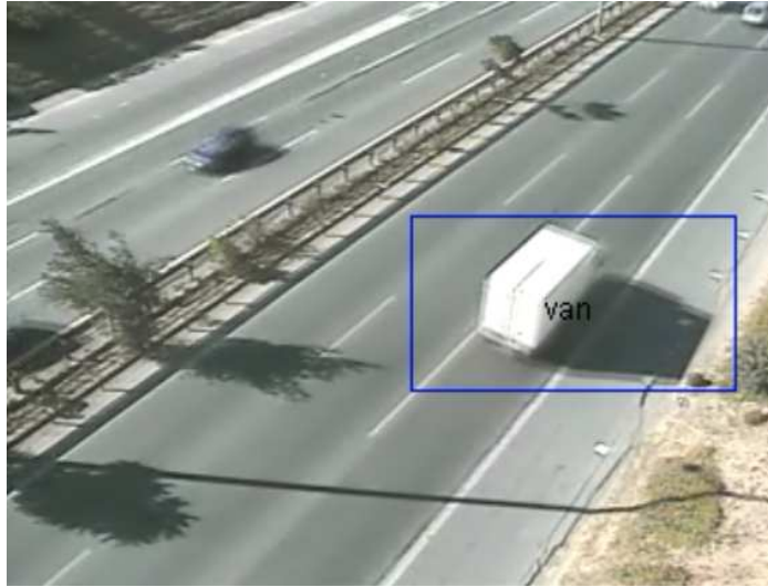
Figure 4.14. An example of incorrect classification when only blob feature used
