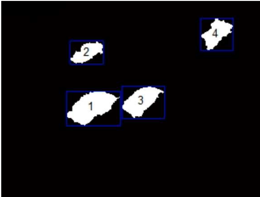
Figure 3.5. Connected component labelling and area filtering on the image
