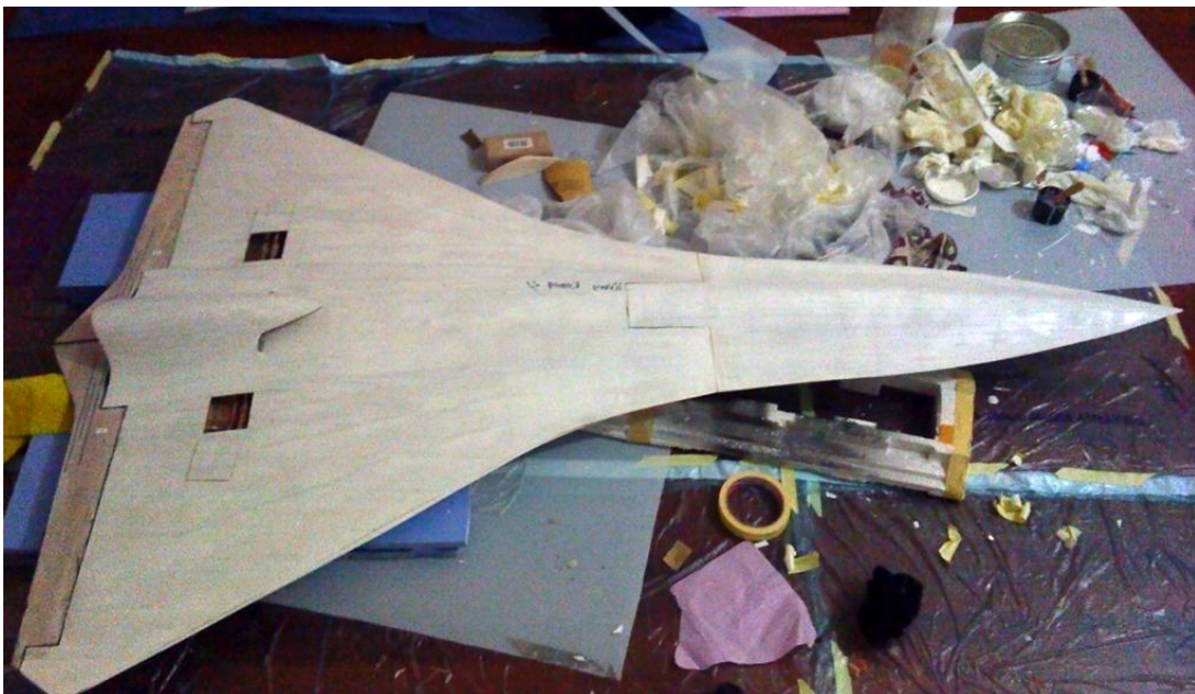
Figure 5. 6 The Surface is applied e-glass and epoxy resin.
