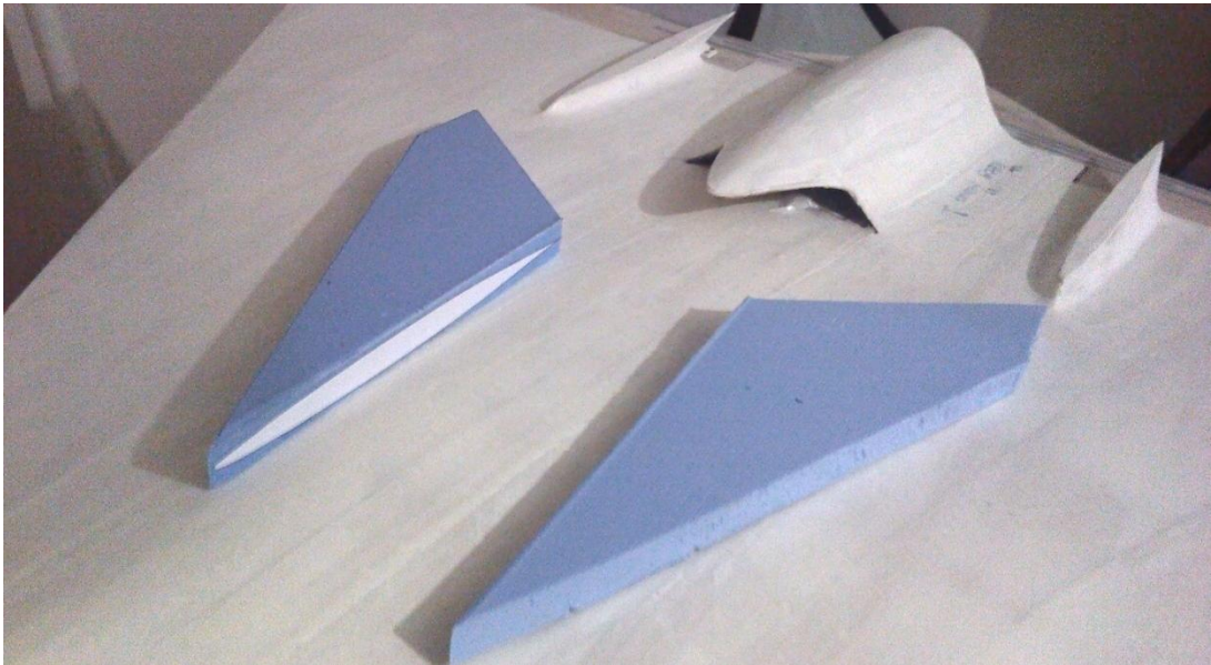
Figure 5.7 The tail blocks before sanding process.
