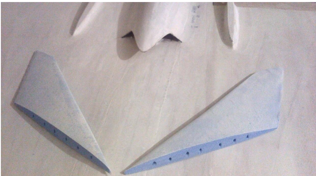
Figure 5.8 The Left and Right Tails after the sanding and fibering process.
