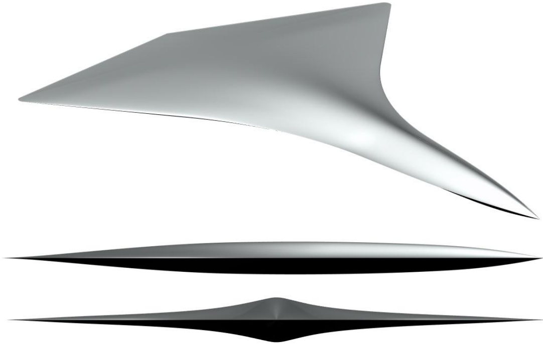
Figure 4. 6 From Up to Bottom; The Isometric, Right and Front View of The Lofted and Joined Upper and Lower Surfaces.
