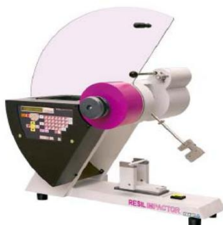
Figure 3.12 The impact testing instrument
