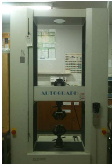
Figure 3.10 The universal tensile testing instrument
