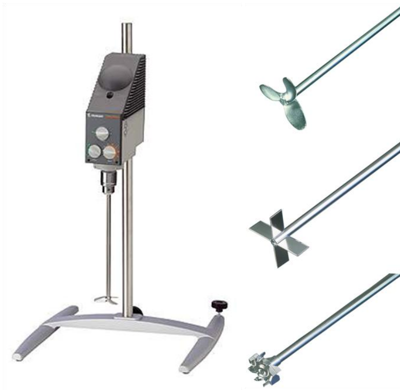
Figure 2.13 Mechanical mixer and some types of impellers [45]
