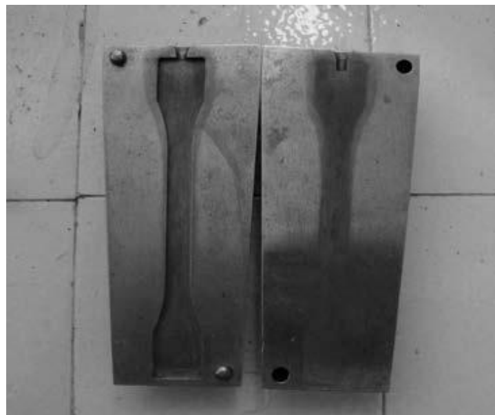
Figure 3.5 – View of the dog-bone mold in the injection molding machine
