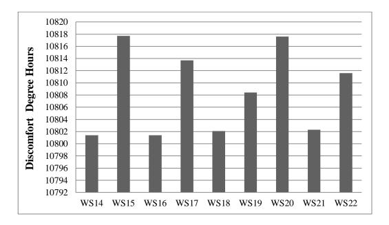
Figure 4.3 Total Yearly Discomfort Degree Hours for South Facing 1.47 m<sup>2</sup> Windows
