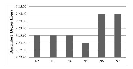
Figure 4.4 Total Yearly Discomfort Degree Hours for North Facing 2.73 m<sup>2</sup> Windows
