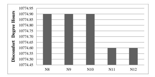
Figure 4.5 Total Yearly Discomfort Degree Hours for North Facing 1.47 m<sup>2</sup> Windows
