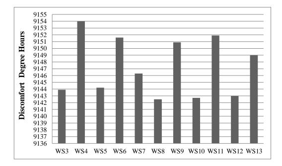
Figure 4.2 Total Yearly Discomfort Degree Hours for South Facing 2.73 m<sup>2</sup> Windows
