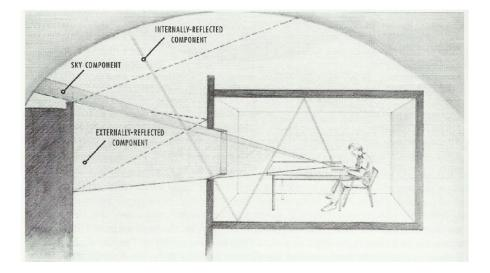
Figure 2.6 Three Components Comprising Daylight Factor (Heerwagen, 2004)
