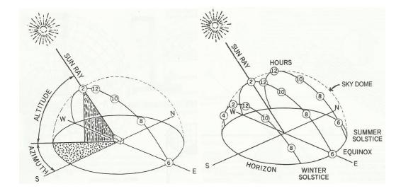
Figure 2.2 Altitude-Azimuth Angles and Three Sun Paths of June 21, September/March 21 and December 21 (Solstices and Equinoxes) (Lechner, 2001)
