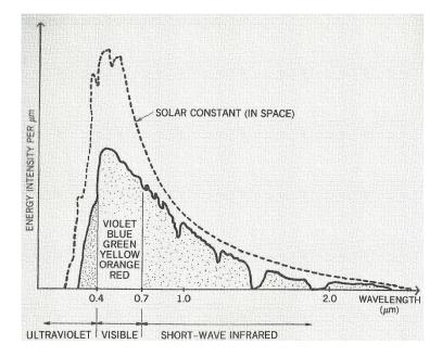
Figure 2.1 The Solar Spectrum (Lechner, 2001)
