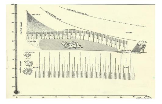
Figure 2.13 Schematic Bioclimatic Chart (Olgyay, 1963)
