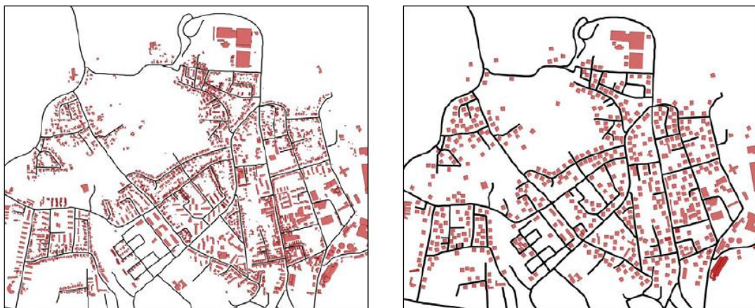
Figure 16 Original data (left), after the typification and displacement (right), (after Hampe and Sester, 2004).
