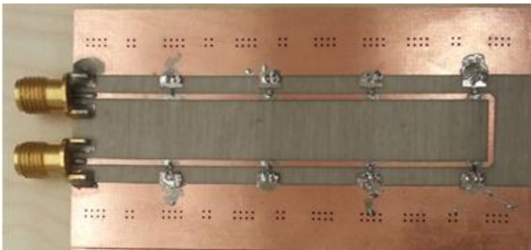
Figure 3-13 Fabricated Eight-Section Loaded-Line Circuit
