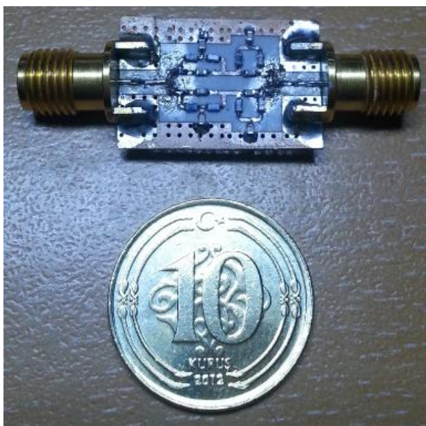
Figure 3-7 Fabricated Two-Stage All Pass Filter Circuit
